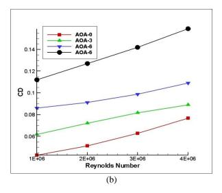
Figure 3:- Variation of drag coefficient with (a) Reynolds Number, (b) Angle of attack
