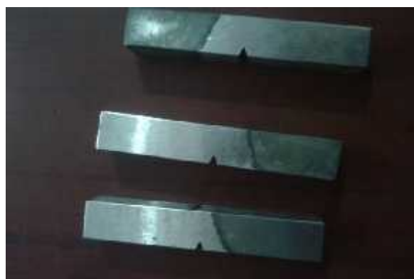
Figure 5:- Charpy Test Specimen
