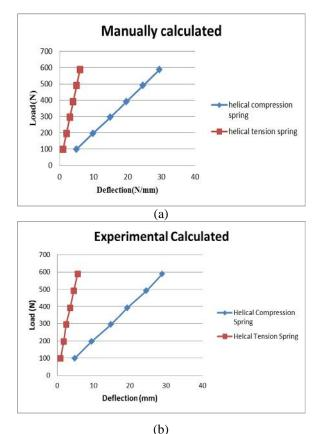
Figure 2:- Variation between load and Deflection for helical compression spring (a) Manually, (b) Experimentally
