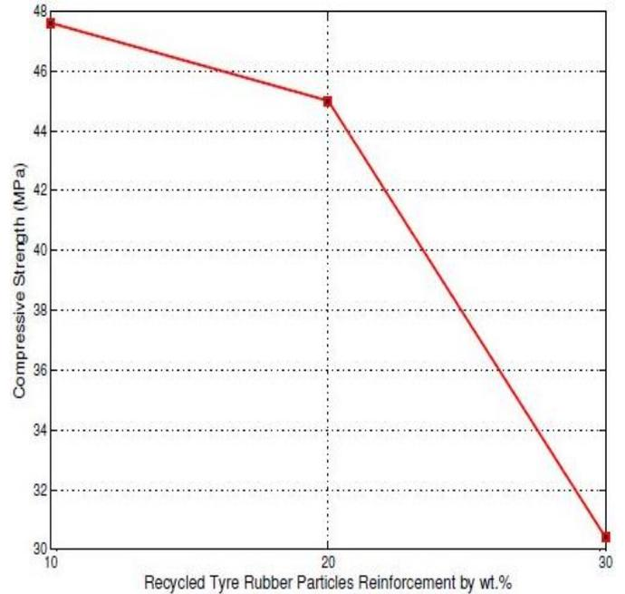
Figure 6: Compressive Strength with variation of tyre rubber particles reinforcement by wt. percentage
