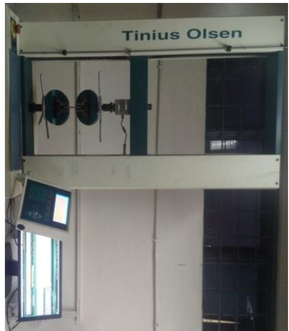
Figure 3.2: Machine used for tensile testing of specimens, Metal Forming Laboratory, D T U, Delhi
