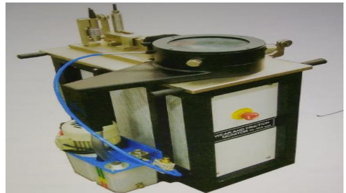
Figure 9: Pin on Disc Wear Testing Machine in DOM Laboratory, DTU
