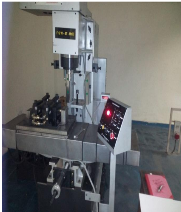
Figure 3.1: Friction stir welding / processing machine ( DTU)
