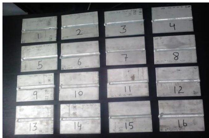
Figure 2: Plate after friction stir welding
