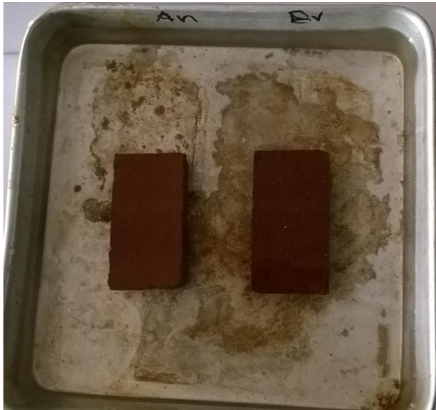
Figure 13. Immersion of bricks in water
