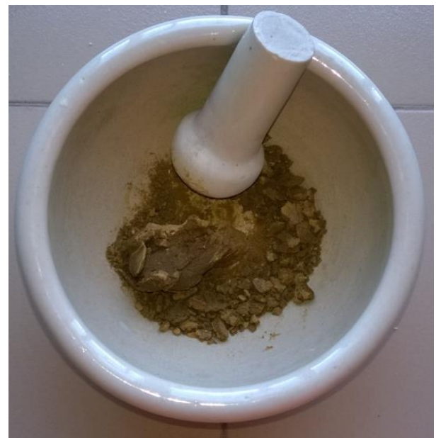
Figure 3. Crushing of dried clay samples
