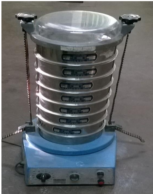
Figure 5. Apparatus setup for sieve analysis
