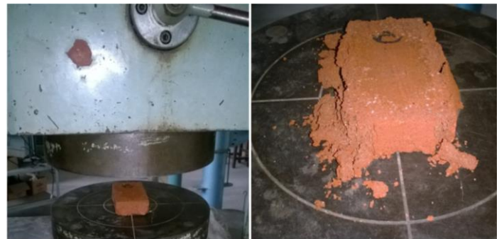
Figure 11. Measuring of compressive load of bricks
