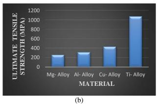
Figure 1: comparison of Mechanical properties (a) Tensile yield strength, (b) Ultimate tensile strength
