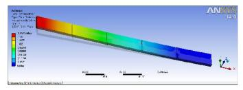
Figure 3 Second mode of vibration
