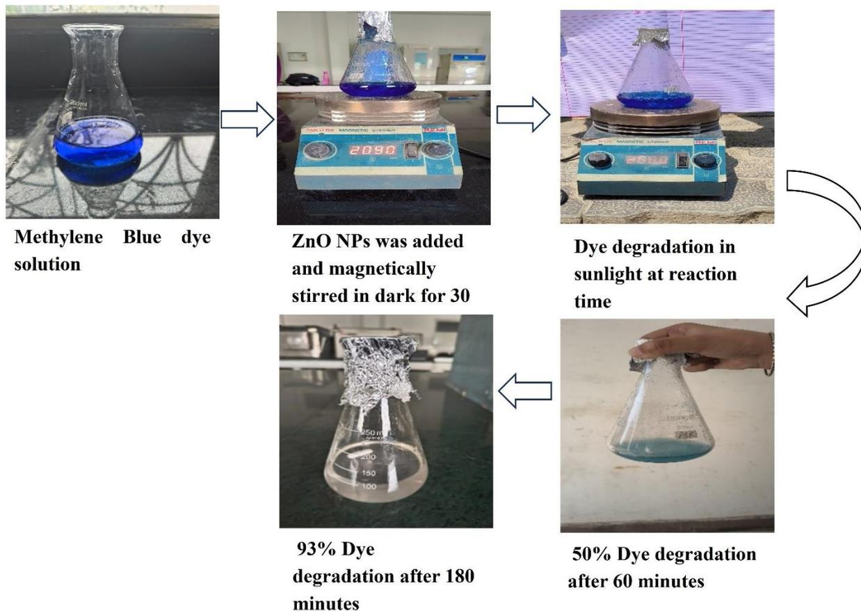
Figure 5: Flowchart of photo-degradation of methylene blue Dye with respect to time
