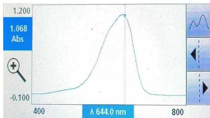
Figure 4: Absorption peak of methylene blue dye
