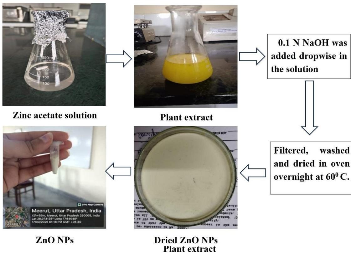
Figure 2: Flow chart of green synthesis of zinc oxide nanoparticles (ZnONPs)
