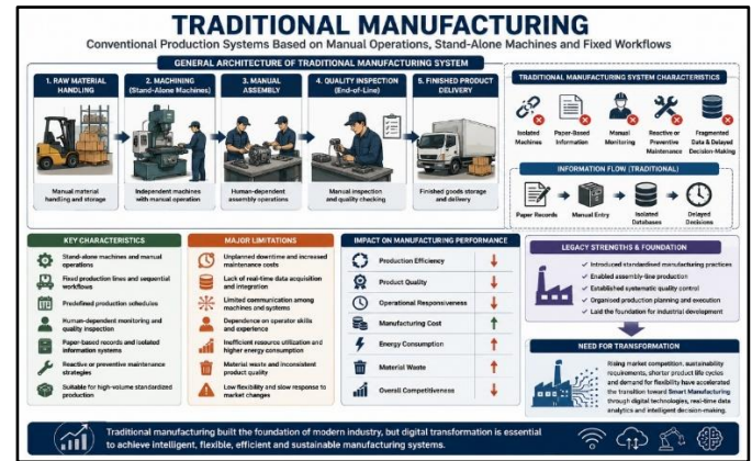
Figure 3: Traditional manufacturing system and its key characteristics [14].
