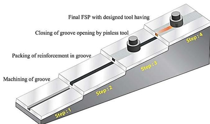
Figure 1. Steps in SCs fabrication using groove technique [33].
