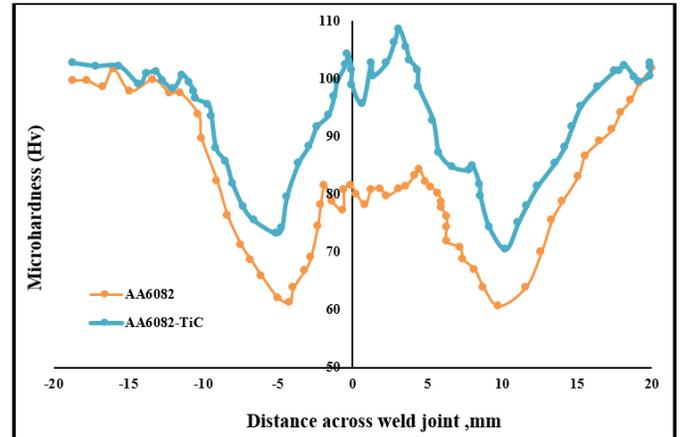
Figure 8: Diagram showing microhardness values of the different specimens [62]
