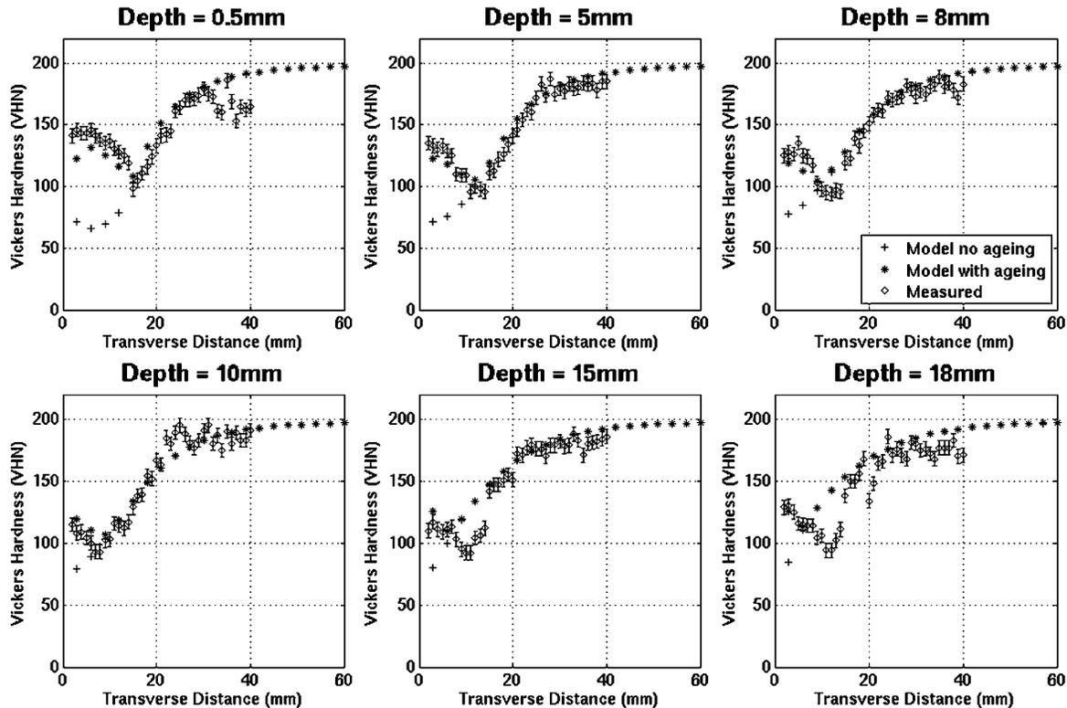
Figure 10: Semi-empirical model predictions and measured hardness profiles in 20 mm thick friction stir weld in 7449-TAF, at six different depths through thickness [65]
