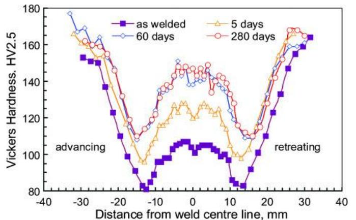
Figure 9: Microhardness variation revealing natural aging in 6 mm 7075-T6 alloy [64]
