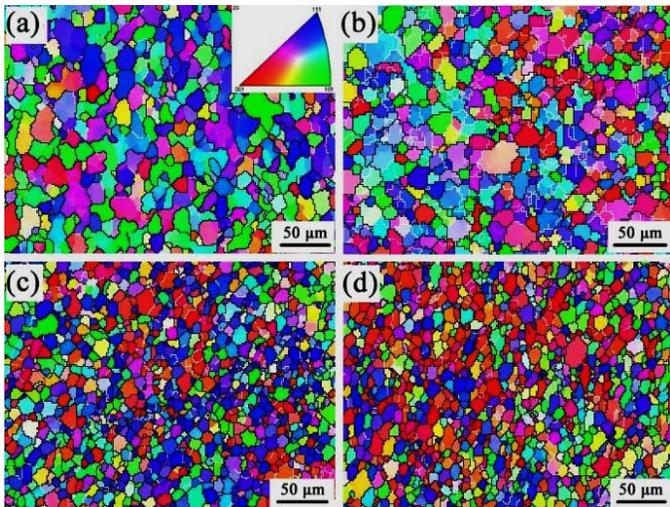
Figure 6: EBSD image at SZ obtained at different TRS (a) 600 rpm, (b) 800 rpm, (c) 1000 rpm and (d) 1200 rpm [60].
