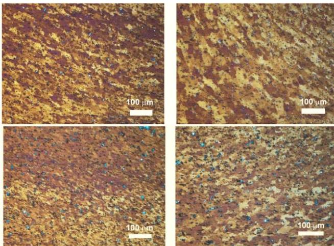
Figure 2: Optical images of friction stir welded joint of AA6082 [54]
