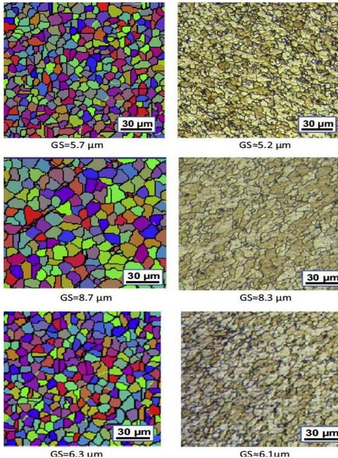
Figure 4: Experimental microstructure of SZ for TRS, TS and shoulder diameter at 900 rpm, 120 mm/min and 16 mm [56]
