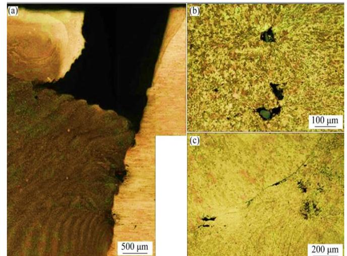
Figure 5: Welding defects formed under different process parameters: (a) 800 r/min, 200 mm/min; (b) 1000 r/min, 300 mm/min; (c) 1400 r/min, 100 mm/min [57]
