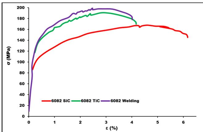
Figure 7: Stress-strain curve for different specimens [61]
