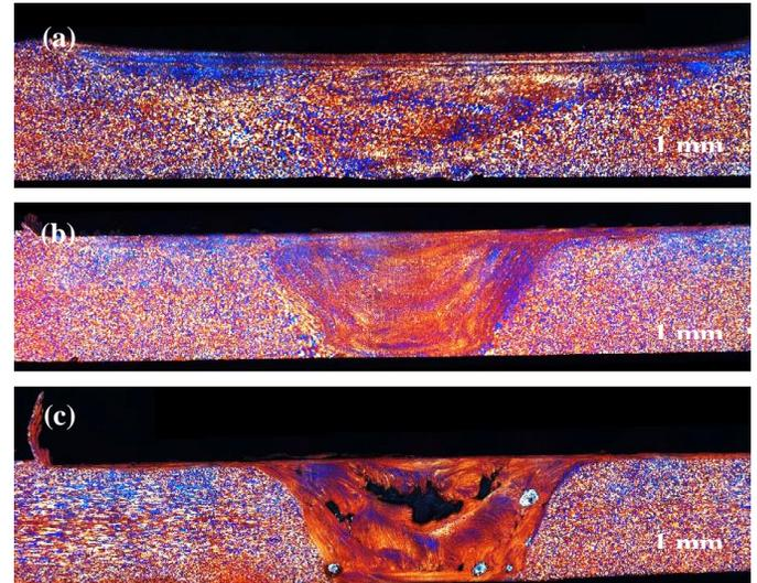
Figure 3: OM image of FSWed joint of AA5754 at (a)  $R = 0$  mm, (b)  $R = 0.5$  mm and (c)  $R = 1$  mm [54].
