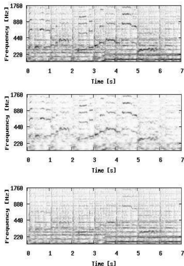
Fig.1. A sample result of two-stage HPSS. Top figure shows the spectrogram of a mixed music signal. Middle figure shows the spectrogram of extracted singing voice by two-stage HPSS. Bottom figure shows the spectrogram of the residual component, i.e., the sum of the ‘harmonic’ and ‘percussive,’ which is roughly equal to the accompaniment.
