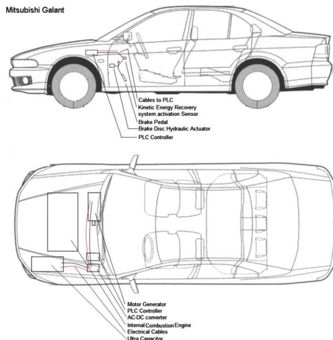
Figure 1: Kinetic energy recovery system overview [8]
