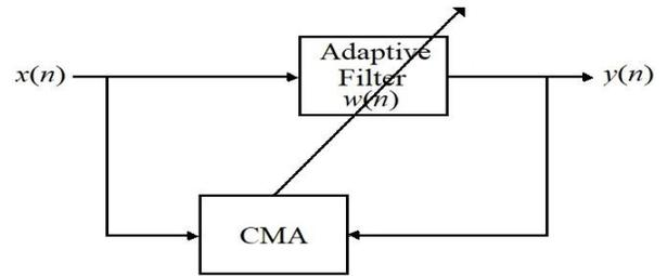
Figure 2: CMA Adaptive Algorithm Block Diagram
