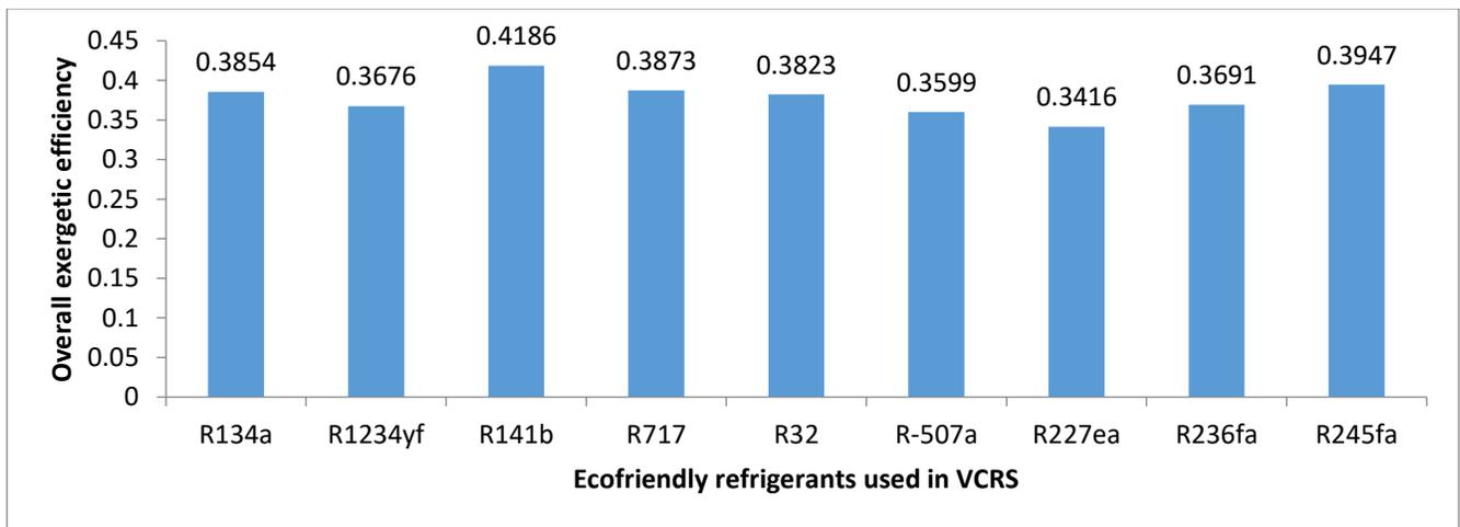
Figure 9: Thermal second law performances (Overall Exergetic Efficiency) of Cascade double effect LiBr Vapour absorption refrigeration system coupled with vapour compression refrigeration using ecofriendly refrigerants in the low temperature cycle of VCRS system
