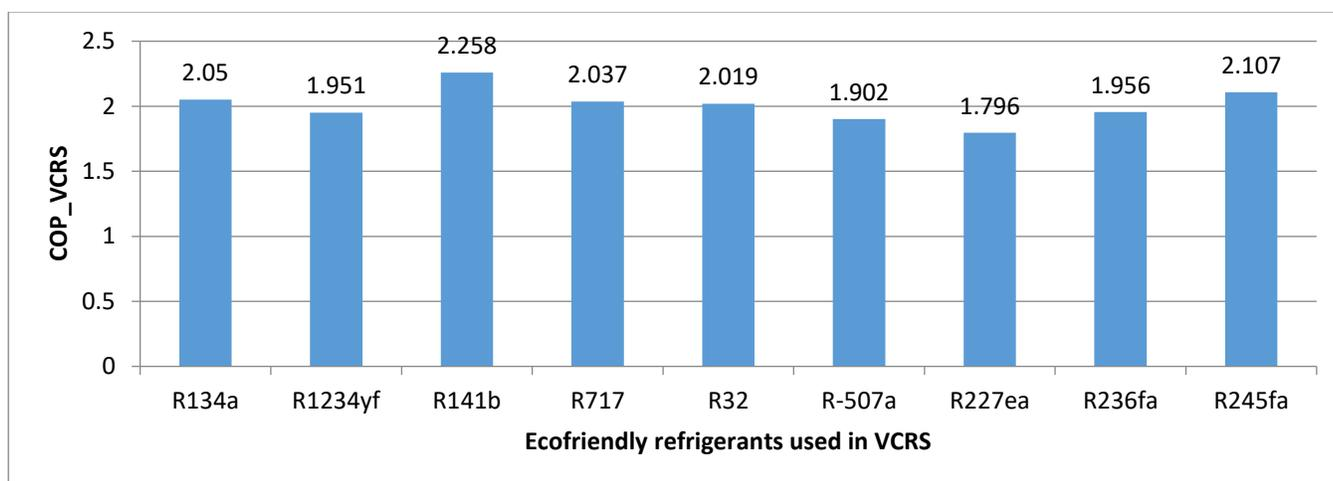
Figure 4: Thermal first law performances (COP\_VCRRS) of cascade triple effect LiBr vapour absorption refrigeration system coupled with vapour compression refrigeration using ecofriendly refrigerants in the low temperature cycle of VCRRS system
