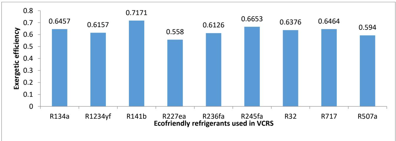
Figure 18: Thermal second law performances(Exergetic Efficiency \_VCERS) of cascade single effect LiBr vapour absorption refrigeration system coupled with vapour compression refrigeration using ecofriendly refrigerants in the low temperature cycle of VCERS system
