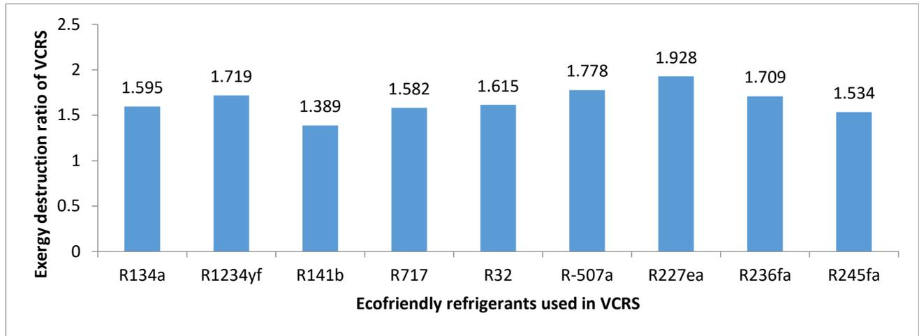
Figure 8: Thermal performances in terms of exergy destruction ratio (EDR\_VCRS) of cascade double effect LiBr Vapour absorption refrigeration system coupled with vapour compression refrigeration using ecofriendly refrigerants in the low temperature cycle of VCRS system
