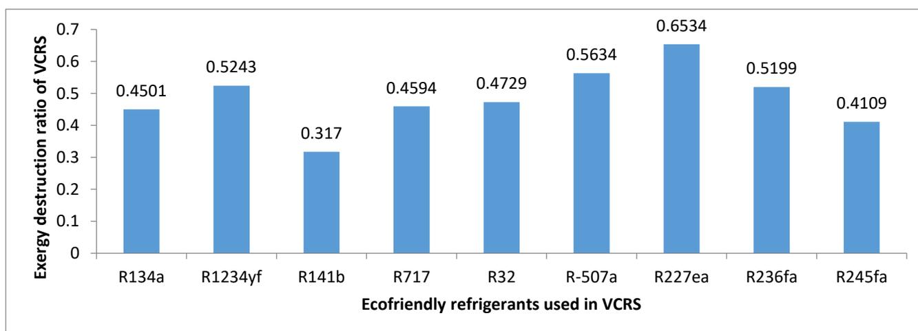
Figure 5: Thermal performances in terms of exergy destruction ratio(EDR\_VCRRS ) of cascade triple effect LiBr vapour absorption refrigeration system coupled with vapour compression refrigeration using ecofriendly refrigerants in the low temperature cycle of VCRRS system
