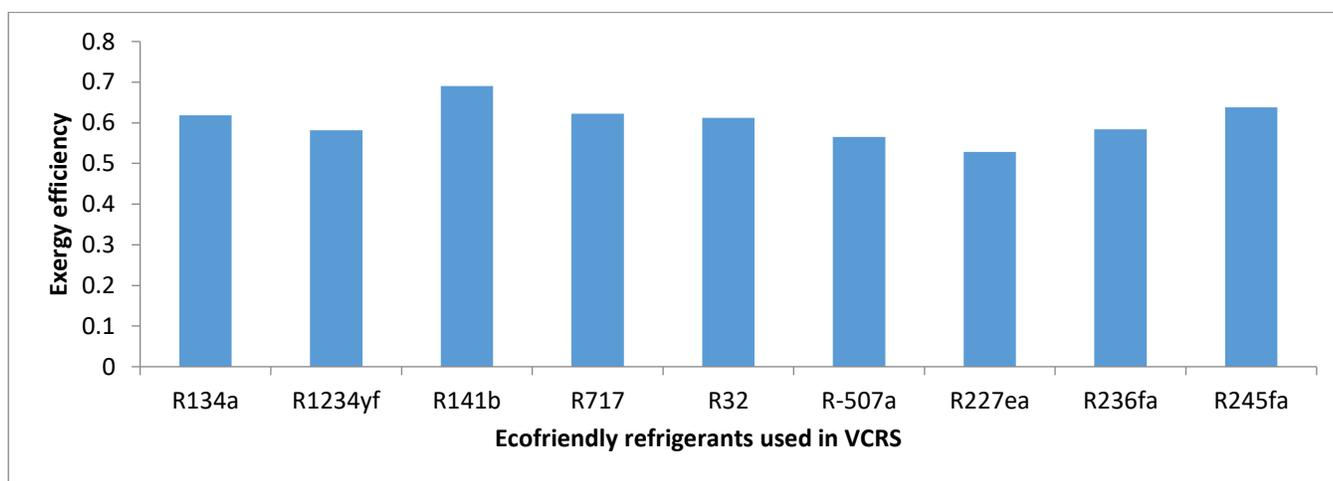
Figure 12: Thermal second law performances (Exergetic Efficiency\_VCRS) of Cascade double Effect LiBr vapour absorption refrigeration system coupled with vapour compression refrigeration using ecofriendly refrigerants in the low temperature cycle of VCRS system
