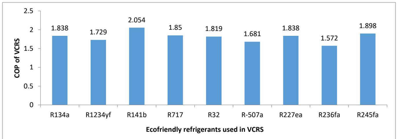
Figure 10: Thermal first law performances (COP\_VCRS) of Cascade double effect LiBr Vapour absorption refrigeration system coupled with vapour compression refrigeration using ecofriendly refrigerants in the low temperature cycle of VCRS system
