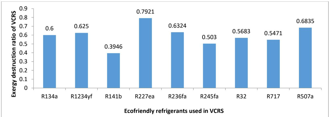
Figure 17: Thermal performances in terms of exergy destruction ratio (EDR\_VCERS ) of cascade single effect LiBr vapour absorption refrigeration system coupled with vapour compression refrigeration using ecofriendly refrigerants in the low temperature cycle of VCERS system
