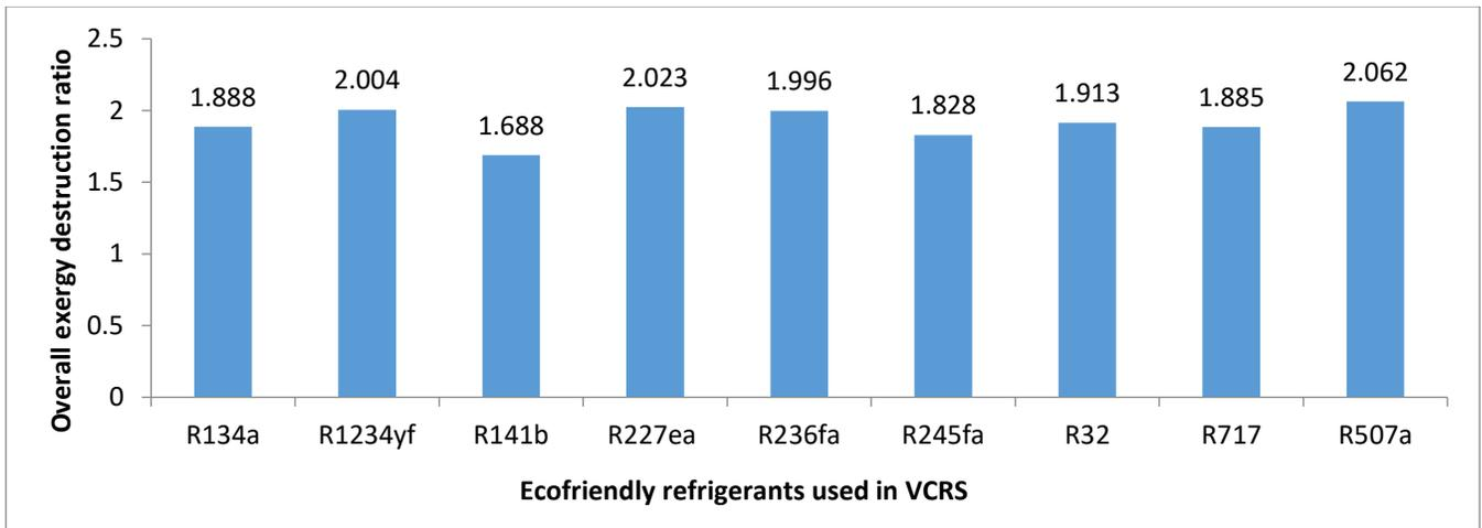
Figure 14: Thermal performances in terms of exergy destruction Ratio ( $EDR_{VCRS}$ ) of cascade single effect LiBr vapour absorption refrigeration system coupled with vapour compression cycle
