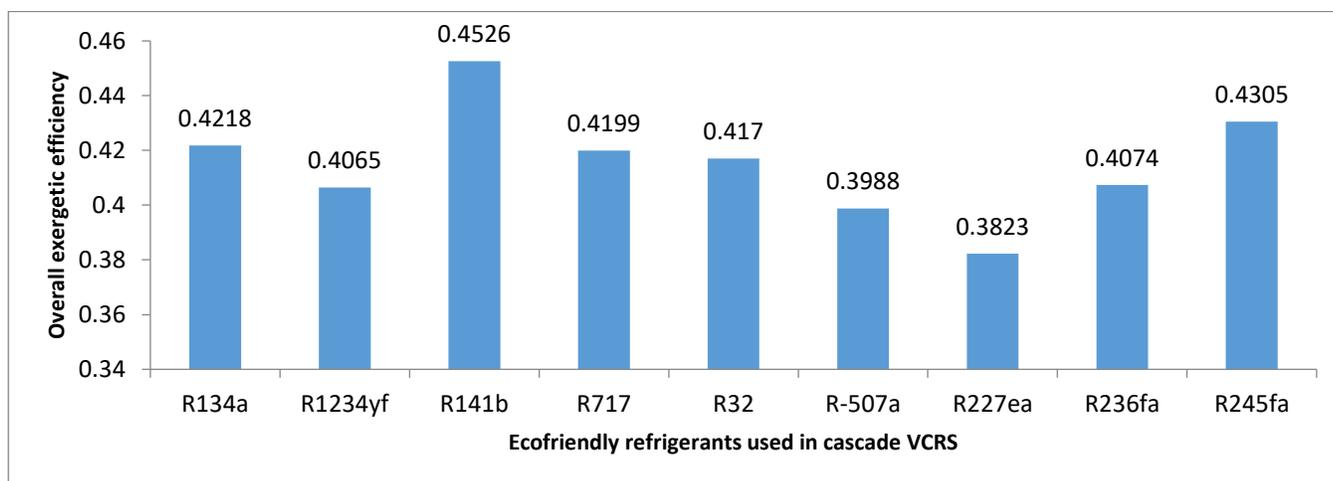
Figure 3: Thermal second law performances (Overall Exergetic Efficiency) of Cascade triple Effect LiBr vapour absorption refrigeration system coupled with vapour compression refrigeration using ecofriendly refrigerants in the low temperature cycle of VCRS system
