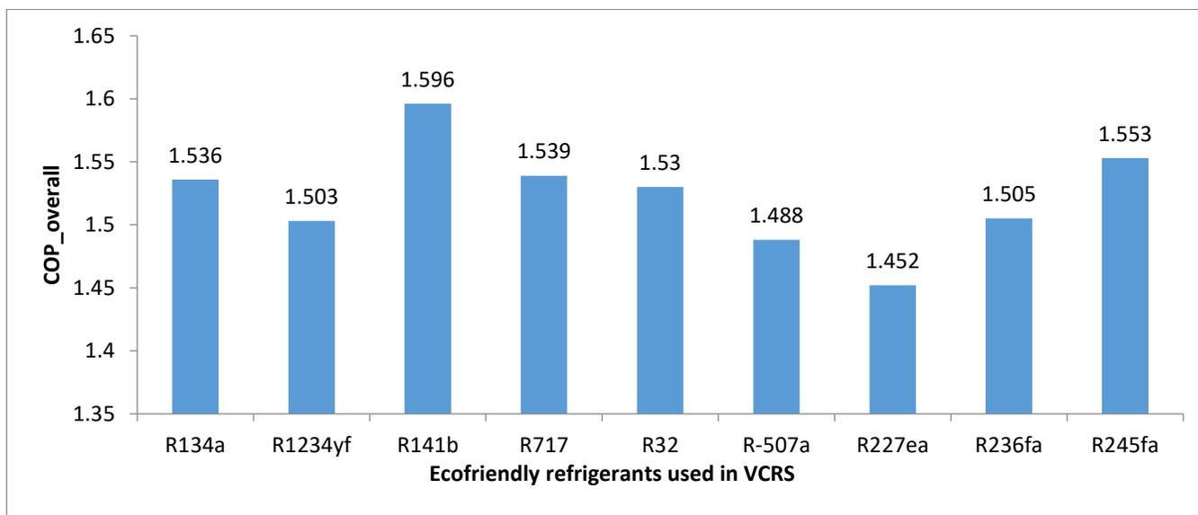
Figure 7: Thermal first law performances (COP\_Overall) of cascade double effect LiBr vapour absorption refrigeration system coupled with vapour compression refrigeration using ecofriendly refrigerants in the low temperature cycle of VCRS system
