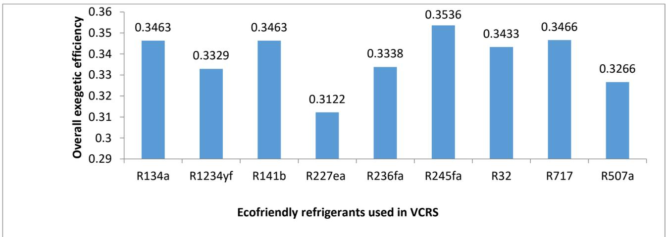
Figure 15: Thermal second law performances ( $Exergetic\ Efficiency_{Overall}$ ) of cascade single effect LiBr vapour absorption refrigeration system coupled with vapour compression refrigeration using ecofriendly refrigerants in the low temperature cycle of VCRS system
