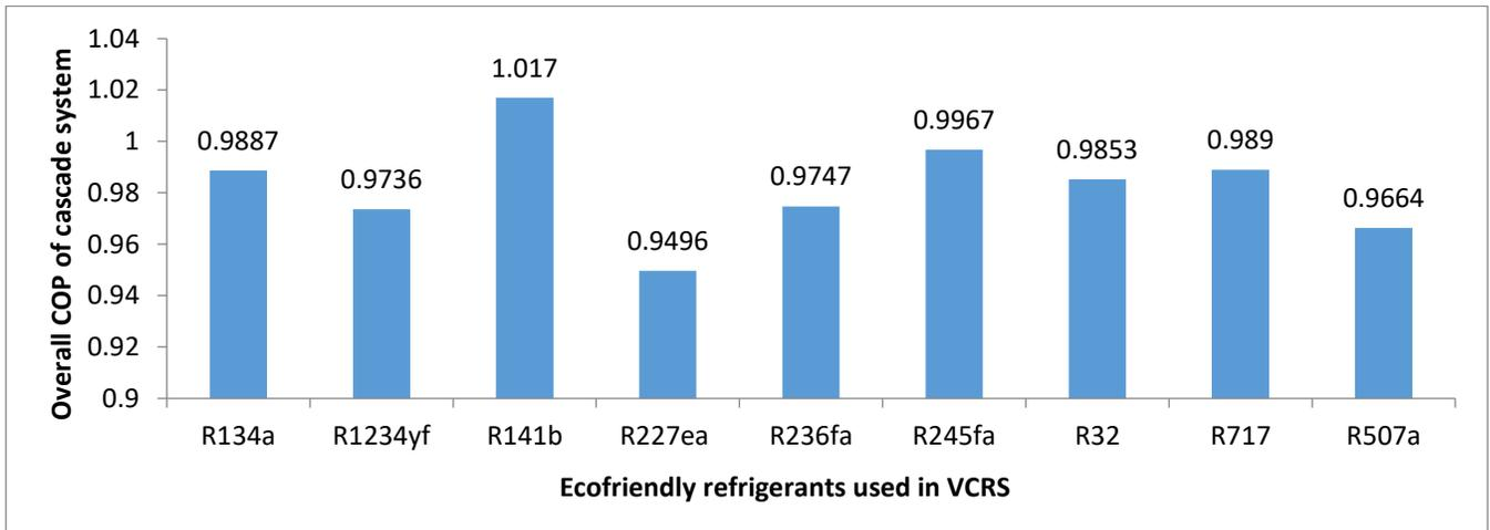
Figure 13: Thermal first law performances ( $COP_{Overall}$ ) of cascade single effect LiBr vapour absorption refrigeration system coupled with vapour compression refrigeration using ecofriendly refrigerants in the low temperature cycle of VCRS system
