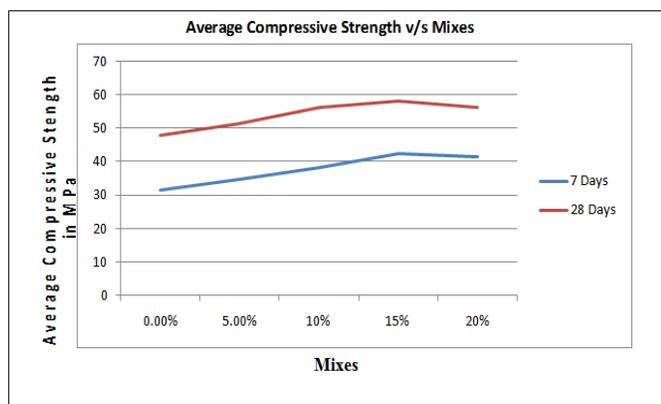
Figure 4: Average compressive strength of concrete v/s Mixes at 7 and 28 days
