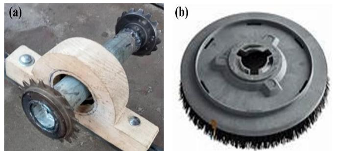
Figure 4: (a) Rolling bearing, (b) Prolite disc brush
