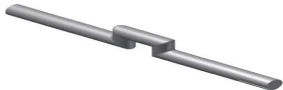
Figure 5: Crankshaft
