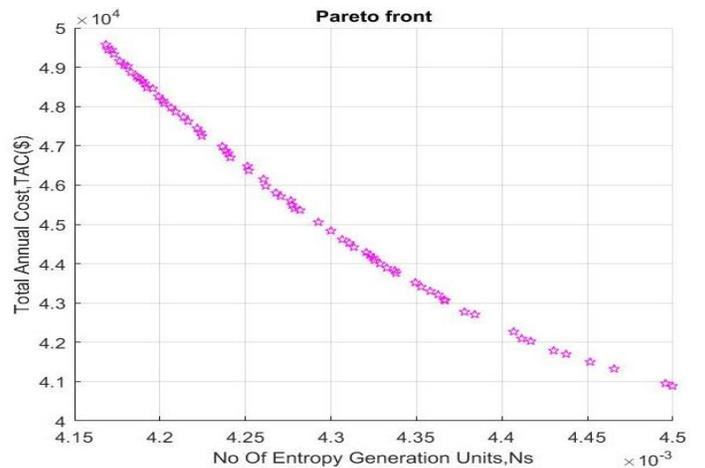
Figure 10: Pareto front for heat transfer constrained case
