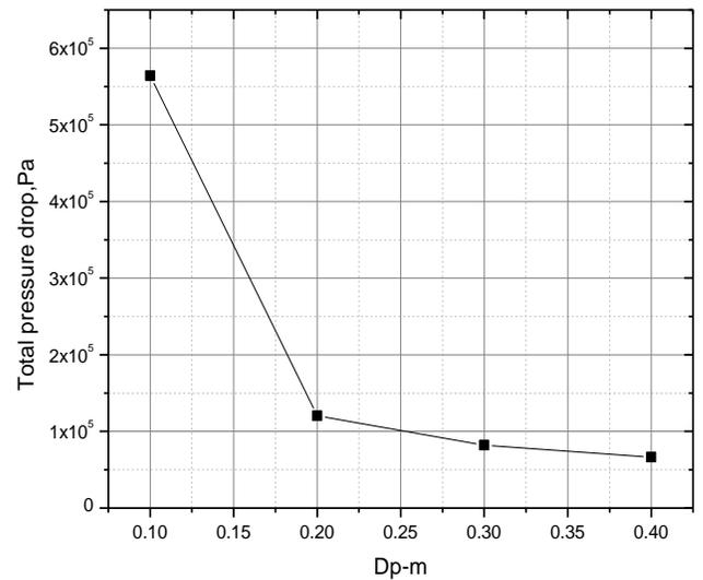
Figure 5: The effect of the horizontal port distance on (a) effectiveness (b) heat transfer (c) total pressure drop
