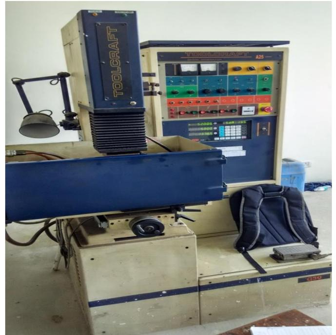
Figure 3 : Electric Discharge Machine, Toolcraft NC machine
