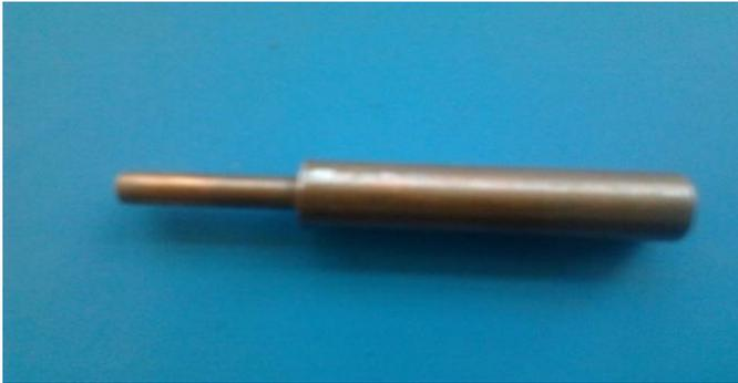
Figure 2: Copper electrode
