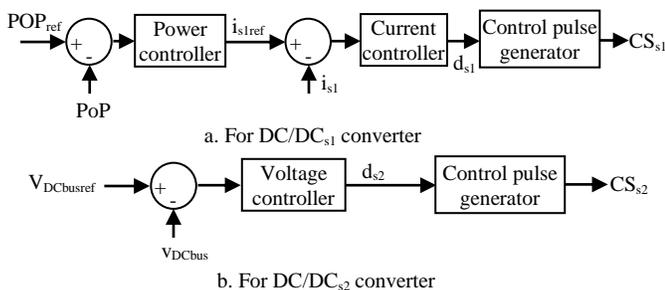
Figure 4: Control structure for DC/DC<sub>s1</sub> and DC/DC<sub>s2</sub> converters
