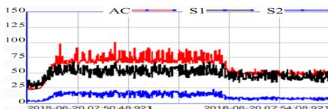
(i) Diagrams of power through DC/AC converter and  $p_{s1}$ ,  $p_{s2}$
