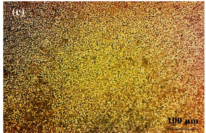
Figure 5: Optical microstructure of multipass FSP/SiC, (b) 1 pass FSP, (c) 3 pass FSP, (d) 5 pass FSP
