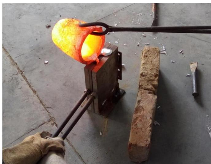
Figure 2: Casting of aluminum alloys
