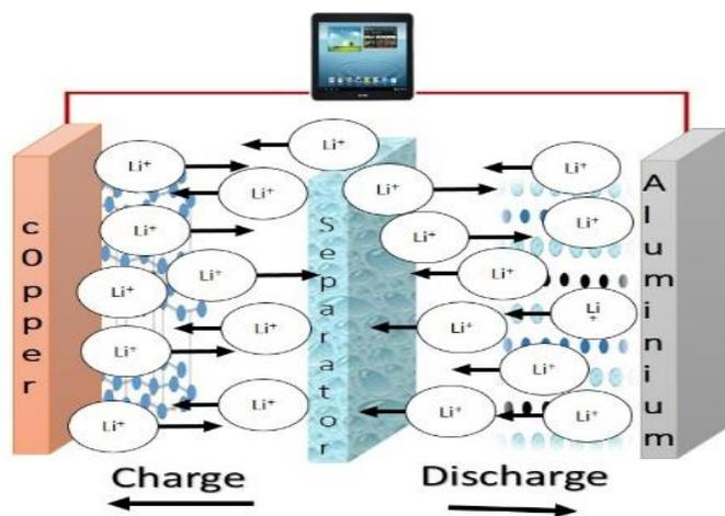
Figure 2: Electrochemical reaction of the Lithium-ion cell during charge and discharge process.
