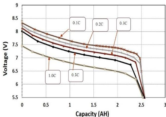
Figure 3: Discharge profiles with different C-rate of the Lithium-ion battery
