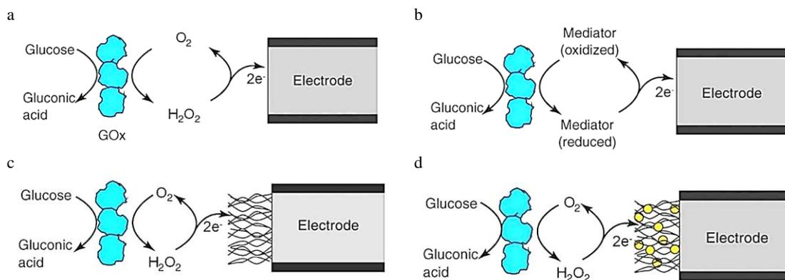
Figure 1: General GOx electrochemical biosensors (a,b). GOx layer (c,d). nanocomposites working together[22]
