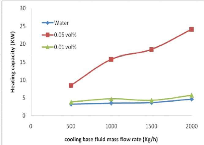
Figure 9: Variation of heating capacity with cooling base fluid mass flow rate (kg.h<sup>-1</sup>)
