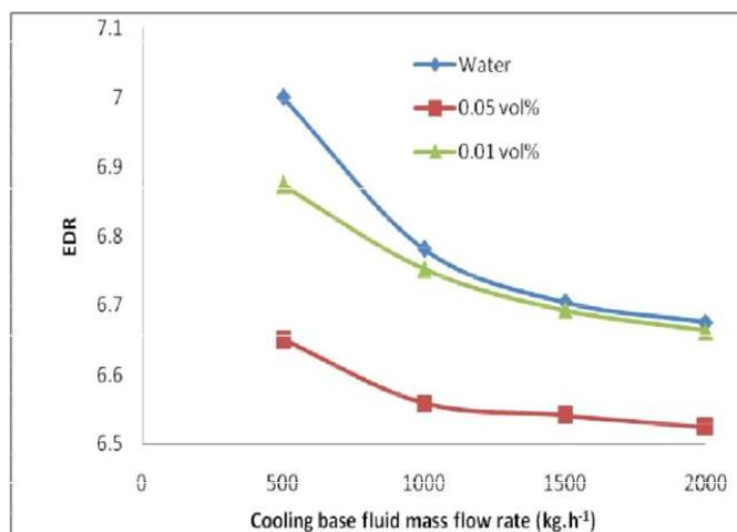
Figure 8: Variation of EDR with cooling base fluid mass flow rate (kg.h<sup>-1</sup>)
