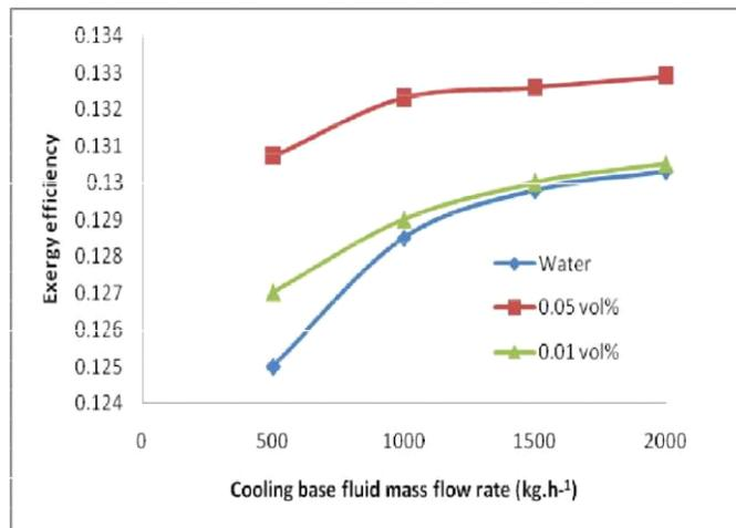
Figure 7: Variation of Exergy efficiency with cooling base fluid mass flow rate (kg.h<sup>-1</sup>)
