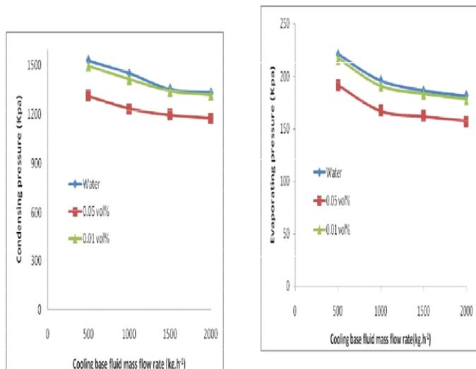
Figure 6: Variation of condensing and evaporator pressures with cooling base fluid mass flow rate (kg.h<sup>-1</sup>)
