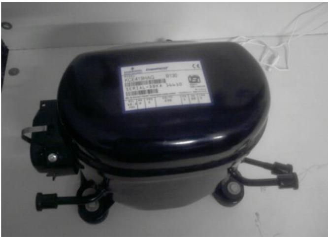
Figure 2: Hermetically sealed reciprocating compressor
