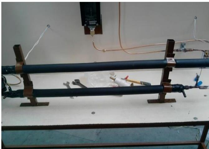
Figure 10: Condenser and evaporator
