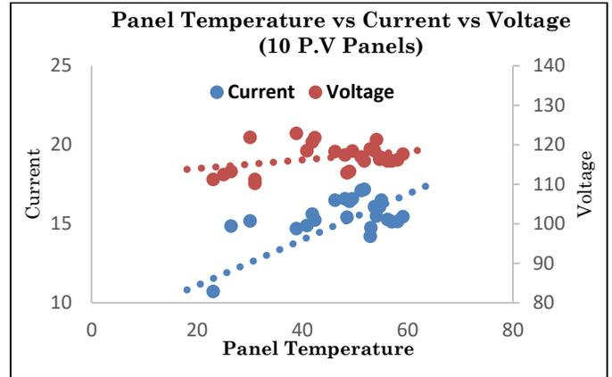
Figure 10: Variation of current and voltage due to panel temperature of 10 P.V panels
