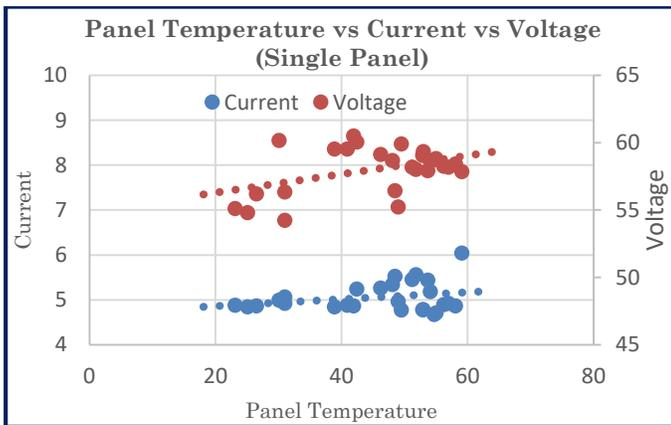
Figure 9: Variation of current and voltage due to panel temperature of a single panel
