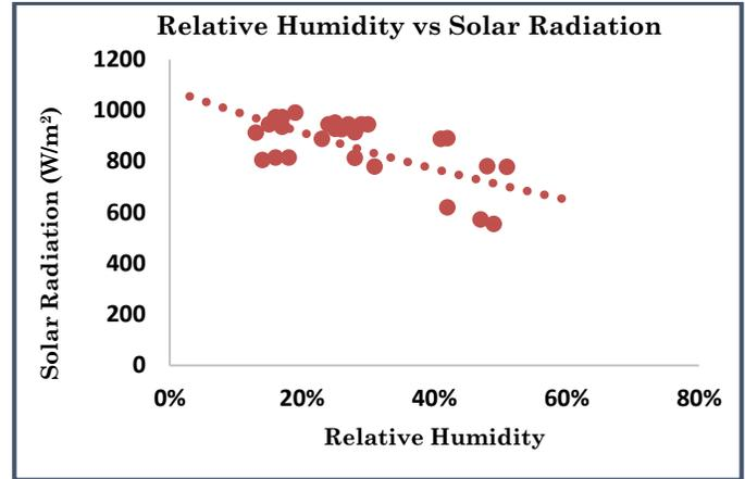
Figure 6: Variation of irradiance level with relative humidity
