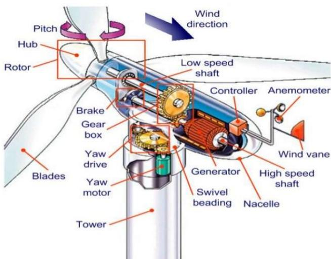
Figure 1: Horizontal wind turbine and its components
