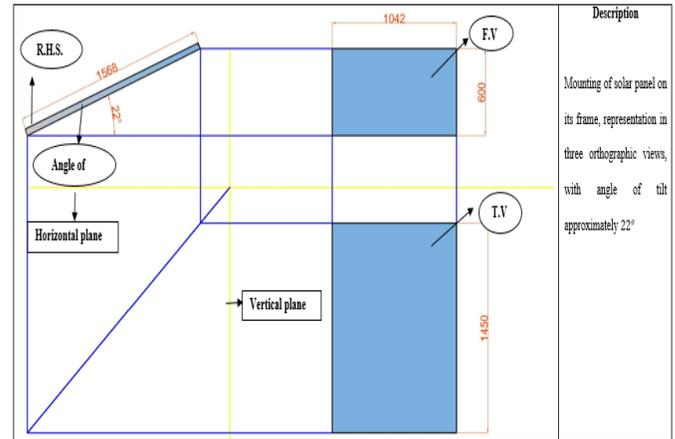
Figure 3: Orthogonal view of a single P.V panel in first angle of projection.
