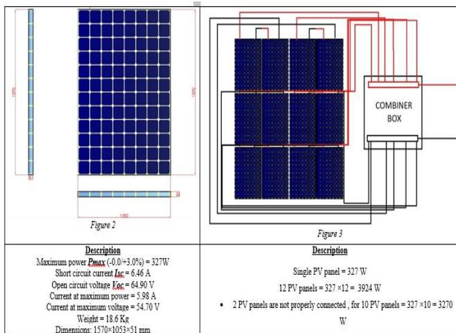
Figure 2: Multi View drawing of Single photovoltaic panel with dimensions and descriptions
