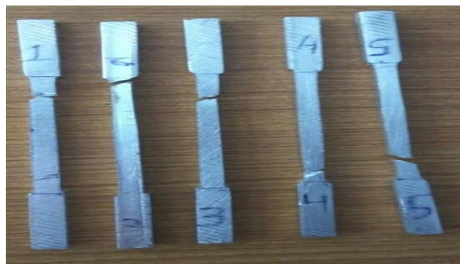
Figure 2: Tensile test specimen after tensile test
