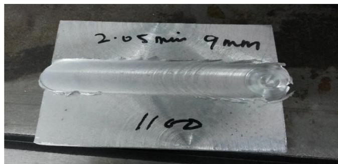
Figure 3: Friction stir welding
