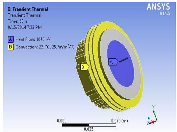
Figure 2: Thermal Loading of the cylinder head
