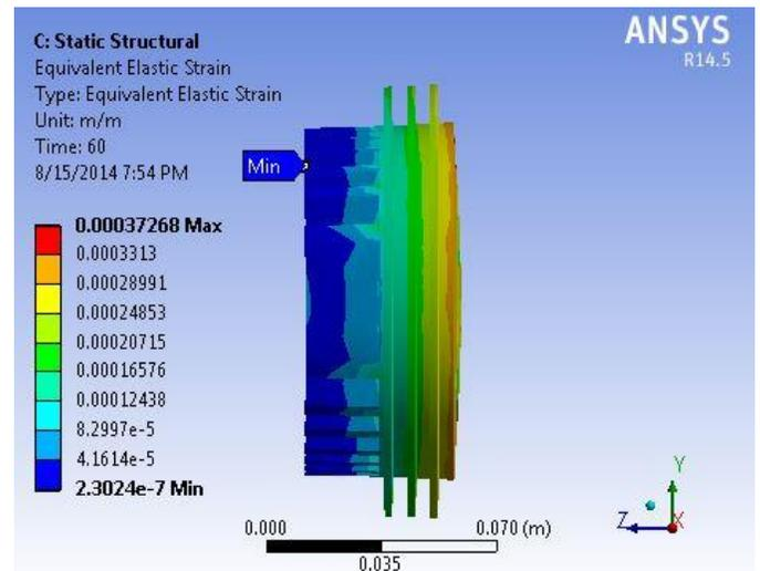
Figure 10: Variation of Thermal Strain with time for the material B390
