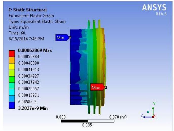
Figure 9: Thermal Strain variation with Time for A380
