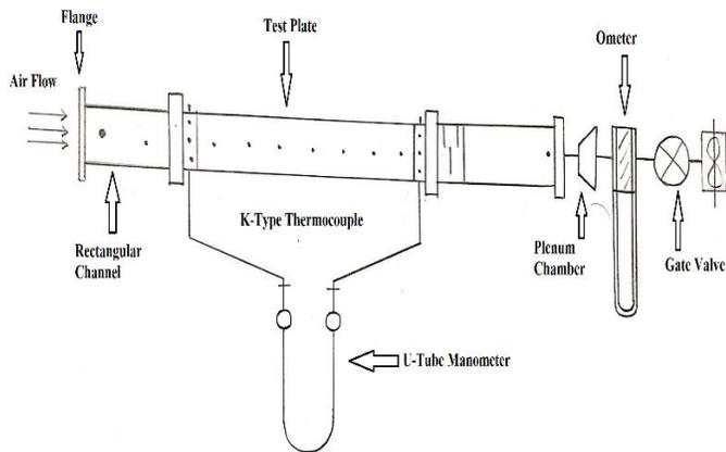
Figure 1: Layout of Test setup
