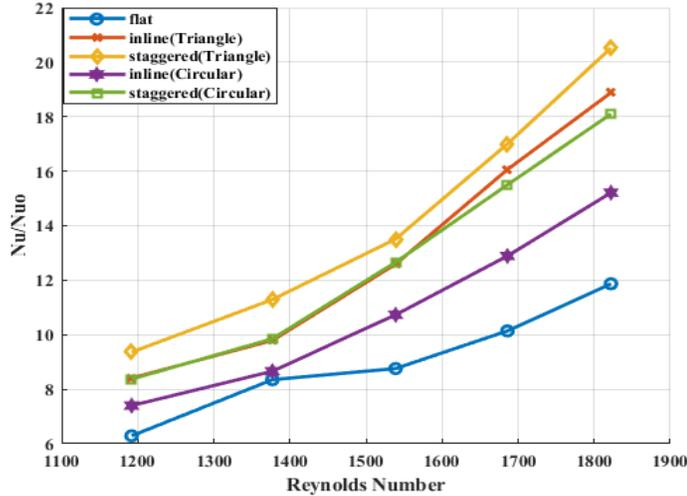
Figure 7: Normalized Nusselt number ratio vs Reynolds number for different dimple Shape.
