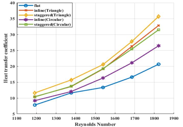
Figure 9 Heat transfer coefficient with different shape of Reynolds number
