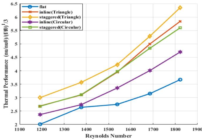
Figure 8: Thermal performance vs Reynolds number for different Shape
