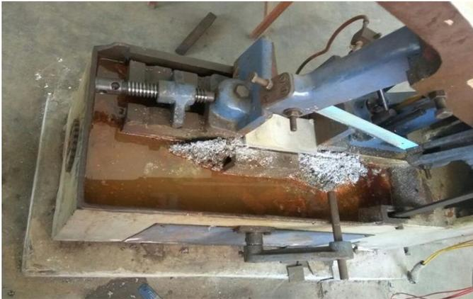
Figure 6: Cutting of base metal plates by power hack saw machine
