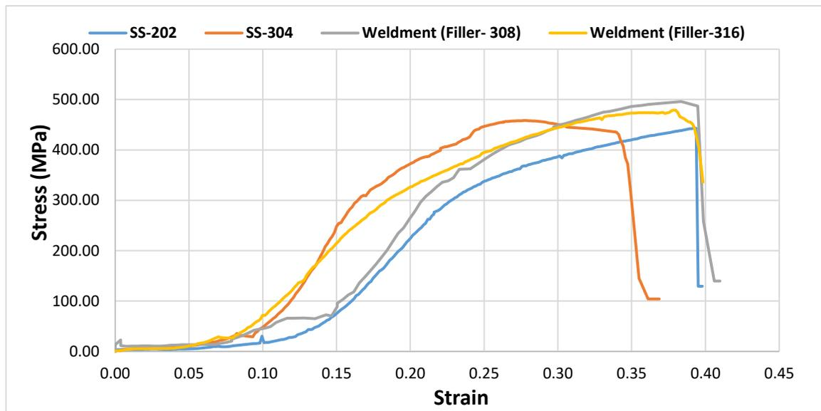
Figure 2: Comparison of Stress strain curve for base material and welded material
