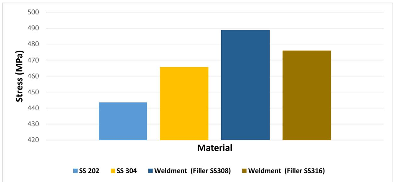
Figure 3: Comparison of Stresses of base material and welded joint by bar graph
