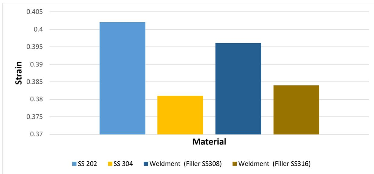
Figure 4: Comparison of Strain of base material and welded joint by bar graph
