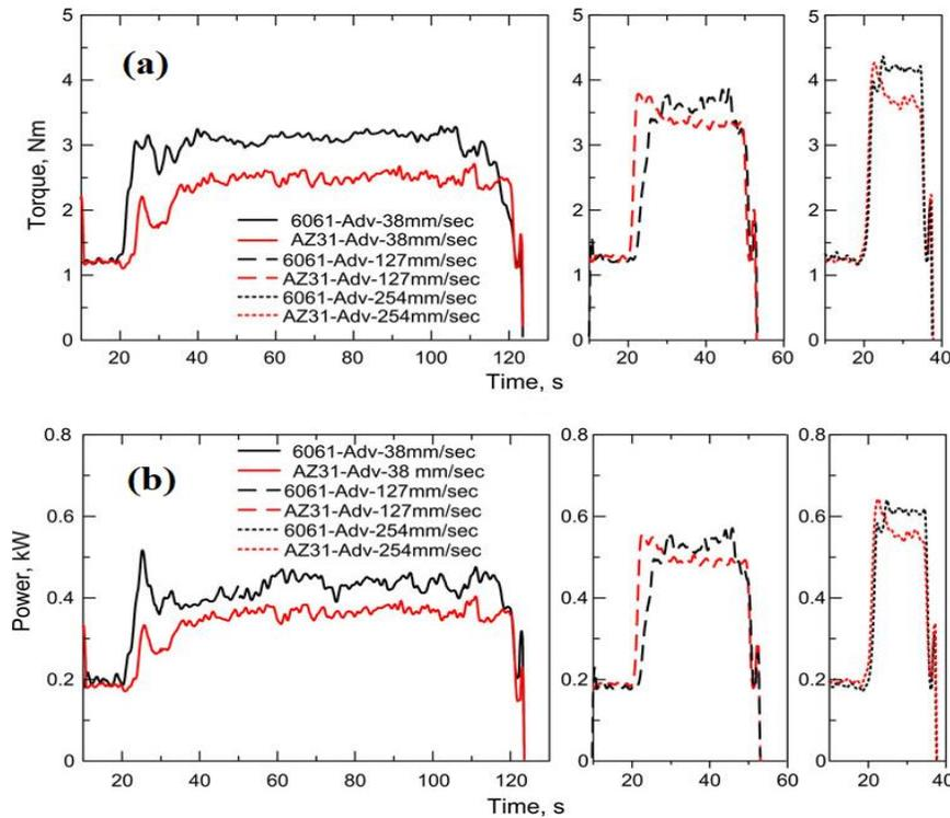
Figure 4. (a) Torque Vs Time graph (b) Power Vs Time of dissimilar FSW of Al 6061 - Mg AZ31B at different travel speeds (in mm/sec) and at rotational speed of 1400rpm [13].
