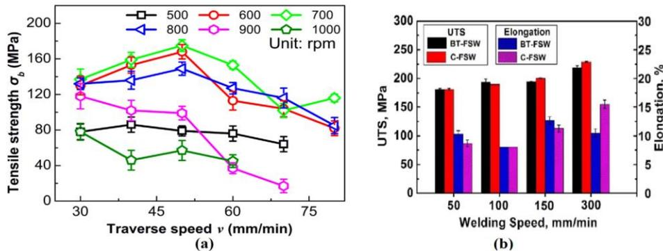
Figure 3: (a) Graph showing variations in tensile strength with increasing welding speed and at constant rotational speed, (b) Graph showing percentage elongation and variation in UTS with increasing welding speed [29, 30].
