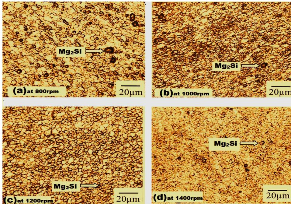
Figure 2: Rotational speed effect on microstructure of Friction stir welding [FSW] zone at different RPMs. (a-d) [23].
