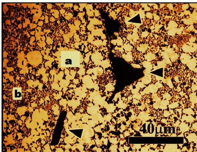
Figure 1: Eutectic microstructure in Al1050 and AZ31 weld performed at  $1.5\text{mm min}^{-1}$  and  $2450\text{ rev min}^{-1}$  [16]
