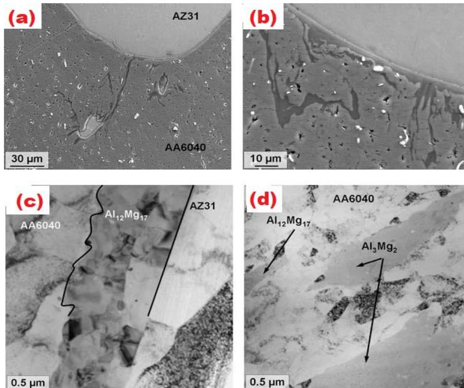
Figure 5. (a) SEM images of Mg alloy AZ31 inclusion in Al alloy AA6040 and IMCs formation around it. (b) Enlarged view of IMCs so formed as described in earlier. (c) TEM image showing the separation of Al alloy AA6040 (left) from Mg alloy AZ31 by fine-grained intermetallic compound (d) TEM image showing the availability of small nano-sized grains of the  $Al_3Mg_2$  phase adjacent to the  $Al_{12}Mg_{17}$  [45]
