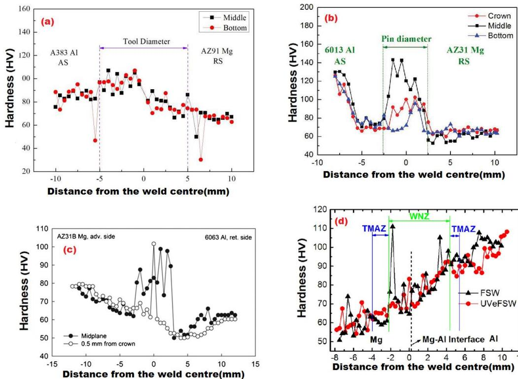
Figure 6: Distribution in hardness level in FSW of Al-Mg:(a)Al-A383 & Mg-AZ91[53];(b)Al-6013 & Mg-AZ31[31];(c)Al-6063&Mg-AZ31B[54];(d)AA 6061-T4 & Mg-AZ31B[55]
