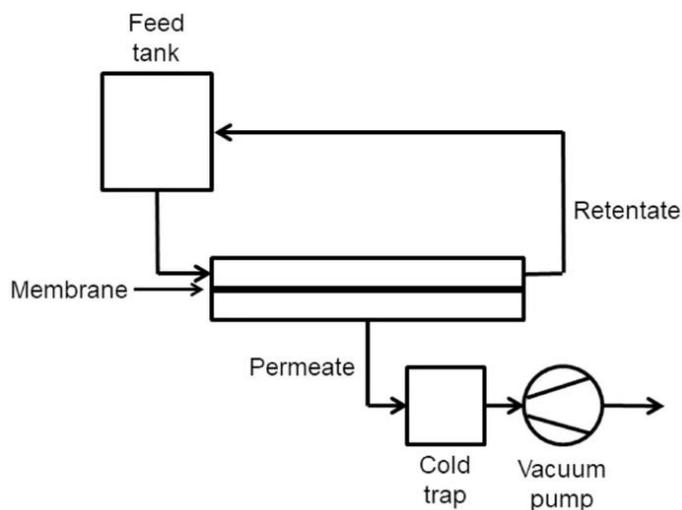
Figure 1: Simplified diagram of pervaporation process
