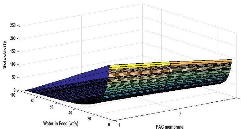
Figure 13: Network Model Prediction for Effect of water concentration in feed on Selectivity
