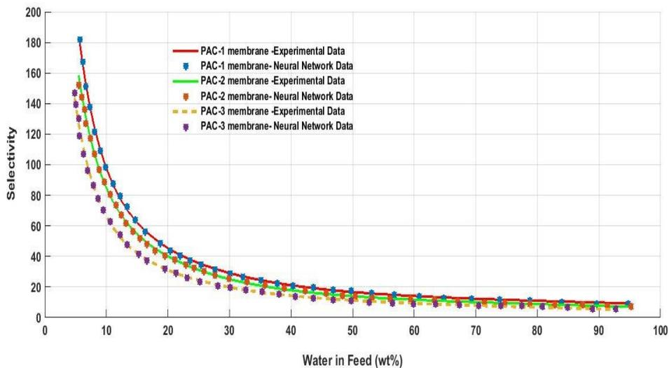
Figure 12: Effect of water in feed concentration on Selectivity (Experimental Data and Network Model Data)
