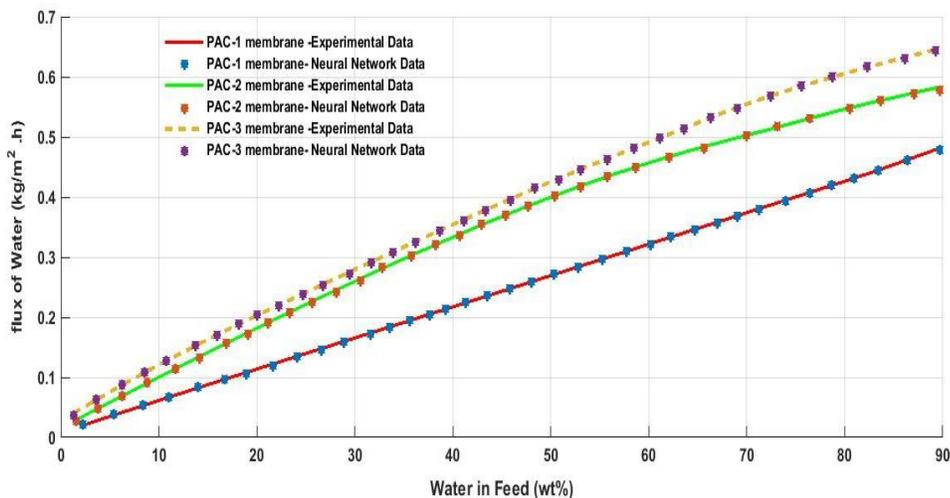
Figure 10: Effect of water in feed concentration on water Flux (Experimental Data and Network Model Data)
