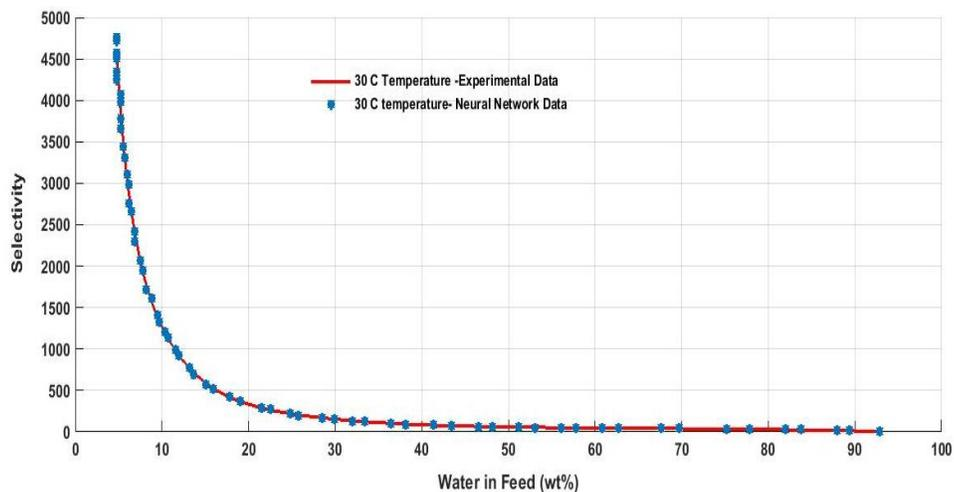
Figure 7: Variation of selectivity of water with feed concentration of water in polyimide membrane at 30°C Polyimide (Experimental Data and Network Model Data)
