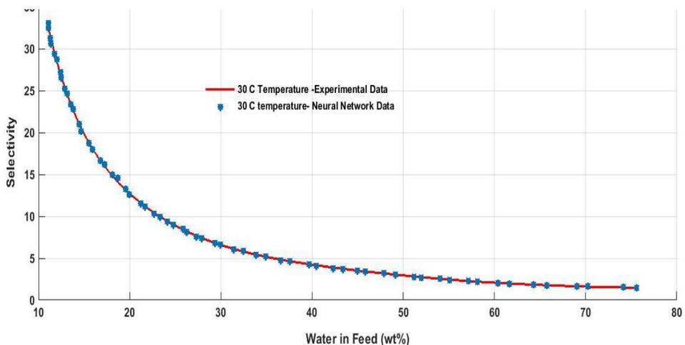
Figure 9: Variation of selectivity of water with feed concentration of water in Nation membrane at 30°C Polyimide (Experimental Data and Network Model Data)
