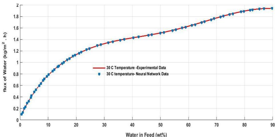
Figure 8: Variation of flux of water with feed concentration of water in Nation membrane at 30°C (Experimental Data and Network Model Data)
