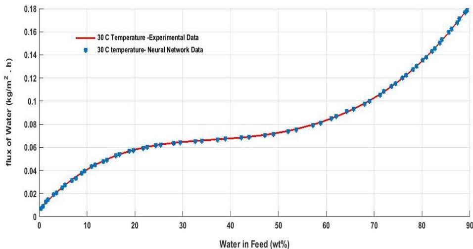
Figure 6: Variation of flux of water with feed concentration of water in polyimide membrane at 30°C (Experimental Data and Network Model Data)
