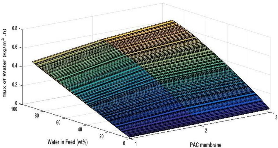
Figure 11: Network Model Prediction for Effect of water concentration in feed on water Flux
