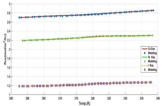
Figure 11: Variation of flux versus temperature for Cs<sup>+</sup>, Sr<sup>2+</sup> and I<sup>-</sup> ionic solutions for a ZSM-5 membrane (Experimental Data and Network Model Data)
