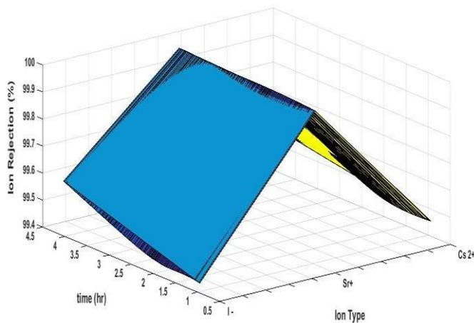
Figure 8: Network Model Prediction for Ion rejection vs. time for ionic solutions through a ZSM-5 membrane Cs<sup>+</sup>; Sr<sup>2+</sup>; I<sup>-</sup>
