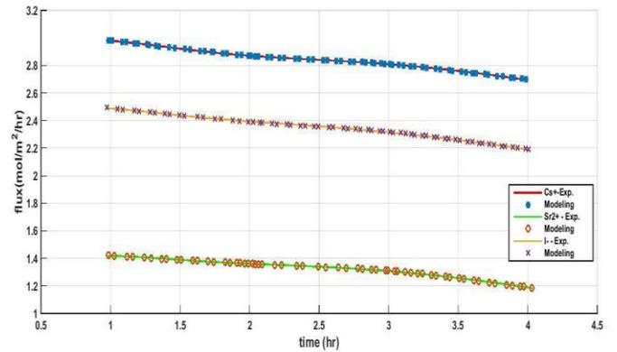
Figure 4. Flux vs. time for ionic solutions through a ZSM-5 membrane Cs+; Sr2+; I- (Experimental Data and Network Model Data)
