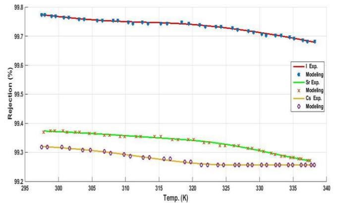
Figure 10: Variation of Ion rejection versus temperature for Cs<sup>+</sup>, Sr<sup>2+</sup> and I<sup>-</sup> ionic solutions for a NaA membrane (Experimental Data and Network Model Data)
