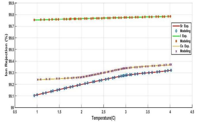
Figure 3. Ion rejection vs. time for ionic solutions through a NaA membrane Cs+; Sr2+; I- (Experimental Data and Network Model Data)
