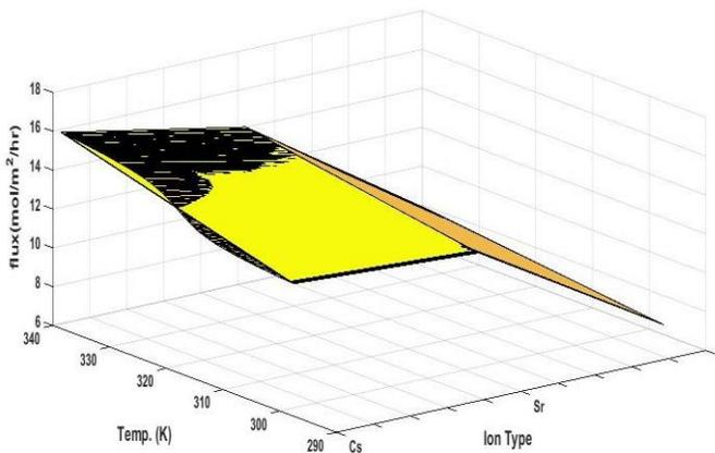
Figure 13: Network Model Prediction flux versus temperature for ionic solutions through a NaA membrane Cs<sup>+</sup>; Sr<sup>2+</sup>; I<sup>-</sup>
