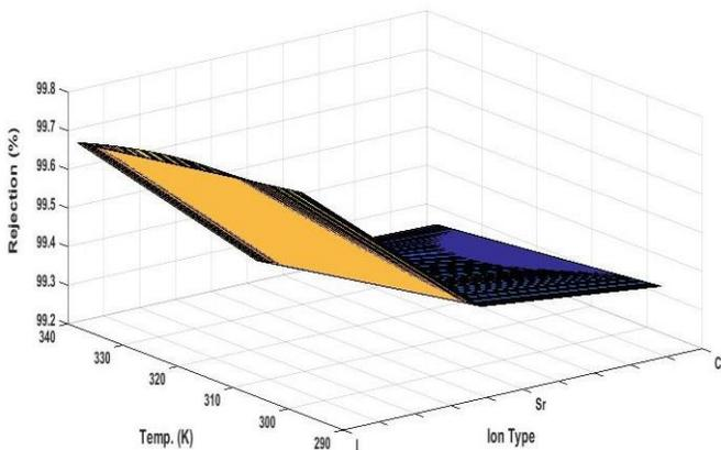
Figure 14: Network Model Prediction Ion rejection versus temperature for ionic solutions through a NaA membrane Cs<sup>+</sup>; Sr<sup>2+</sup>; I<sup>-</sup>
