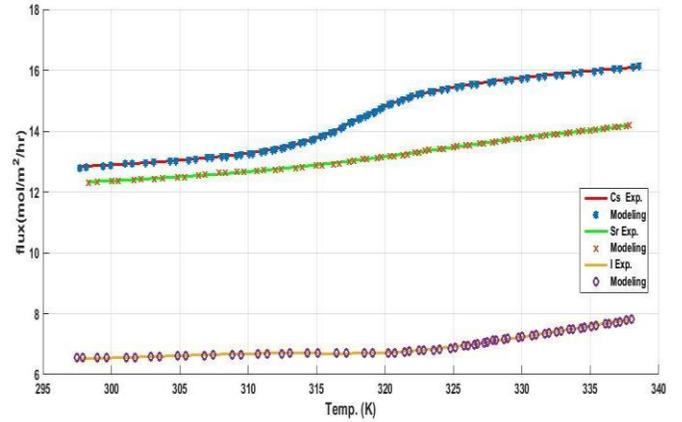
Figure 9: Variation of flux versus temperature for Cs<sup>+</sup>, Sr<sup>2+</sup> and I<sup>-</sup> ionic solutions for a NaA membrane (Experimental Data and Network Model Data)
