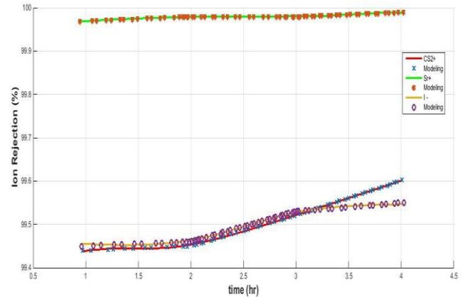
Figure 5. Ion rejection vs. time for ionic solutions through a ZSM-5 membrane Cs+; Sr2+; I- (Experimental Data and Network Model Data)
