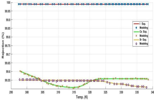
Figure 12. Variation of Ion rejection versus temperature for Cs+, Sr<sup>2+</sup> and I<sup>-</sup> ionic solutions for a ZSM-5 membrane (Experimental Data and Network Model Data)
