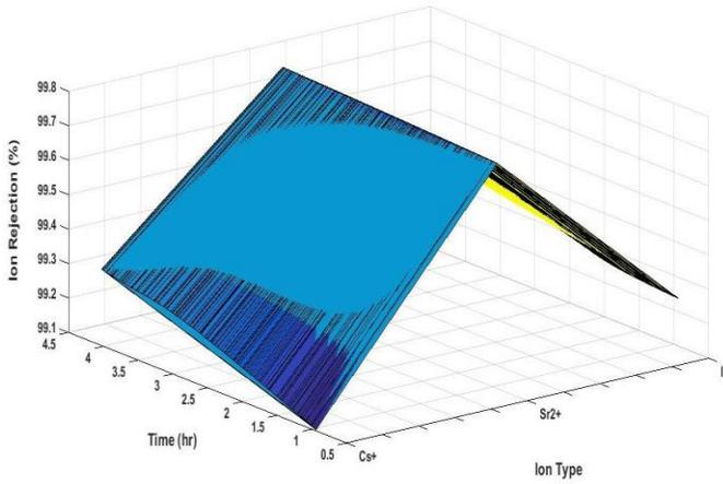
Figure 6: Network Model Prediction for Ion rejection vs. time for ionic solutions through a NaA membrane Cs<sup>+</sup>; Sr<sup>2+</sup>; I<sup>-</sup>
