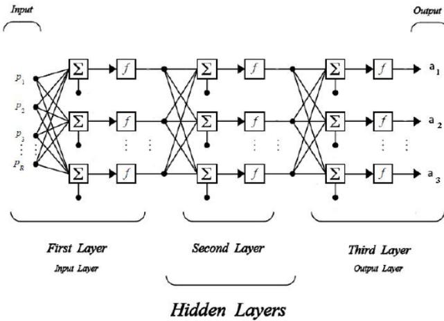
Figure 1. Image of a neural network with its constituent layers
