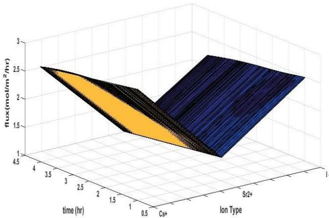
Figure 7: Network Model Prediction for Flux vs. time for ionic solutions through a ZSM-5 membrane Cs<sup>+</sup>; Sr<sup>2+</sup>; I<sup>-</sup>
