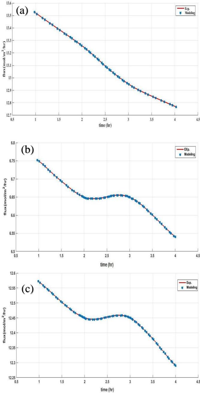
Figure 2. Flux vs. time for ionic solutions through a NaA membrane a) Cs+; b) Sr2+; c) I- (Experimental Data and Network Model Data)
