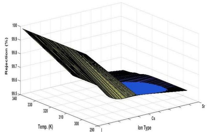
Figure 16: Network Model Prediction Ion rejection versus temperature for ionic solutions through a ZSM-5 membrane Cs<sup>+</sup>; Sr<sup>2+</sup>; I<sup>-</sup>
