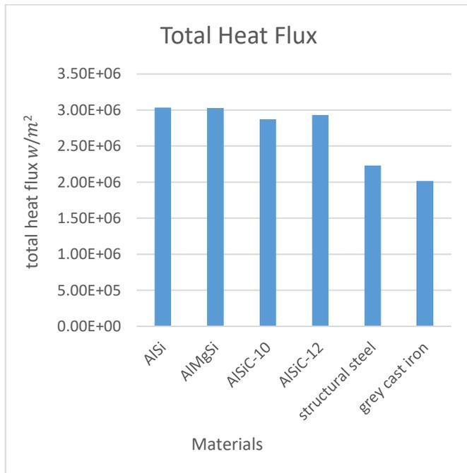
Figure 7: Comparison of Heat Flux for different material
