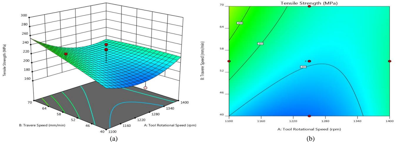
Figure 4: Effect of tool rotational speed and traverse speed on tensile strength of friction stir welded joint
