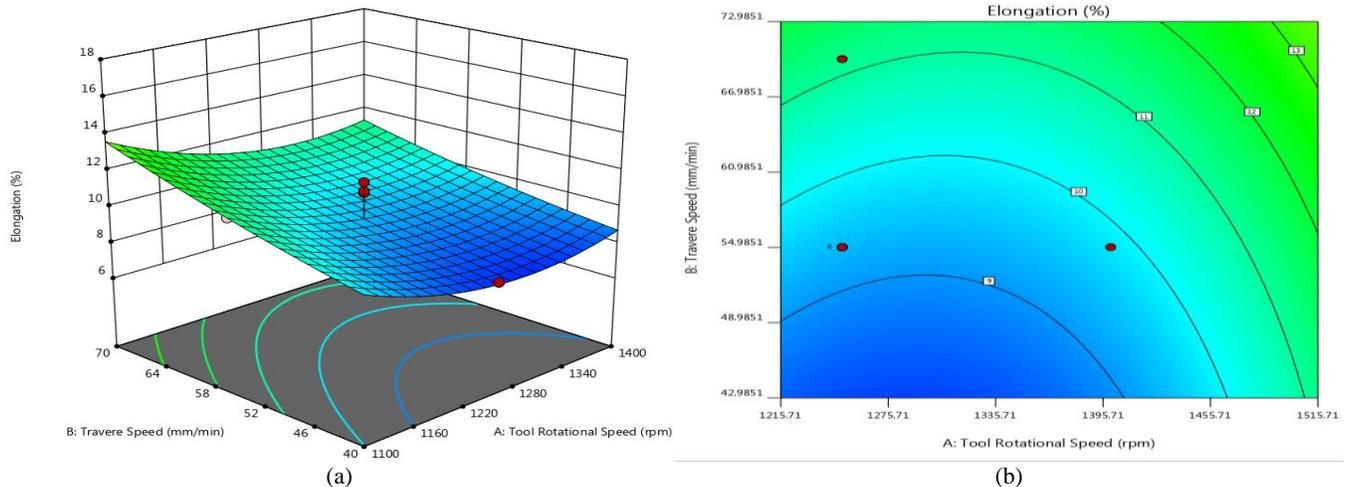
Figure 5: Effect of tool rotational speed and traverse speed on % elongation of friction stir welded joint
