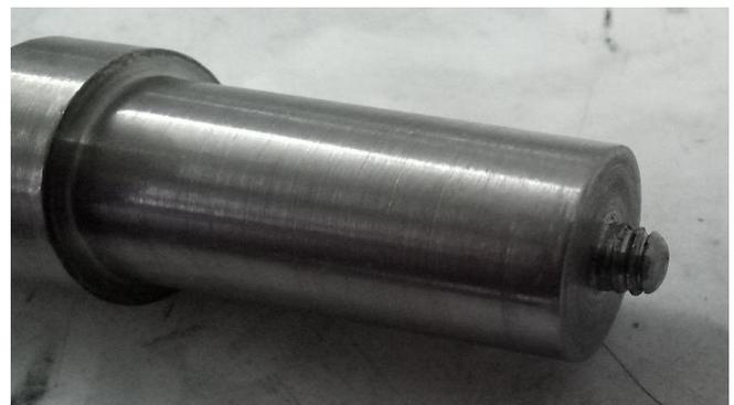
Figure 3: Friction stir welding tool of H13 tool steel
