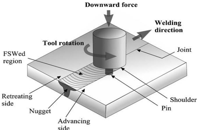
Figure 1: The friction stir welding proces
