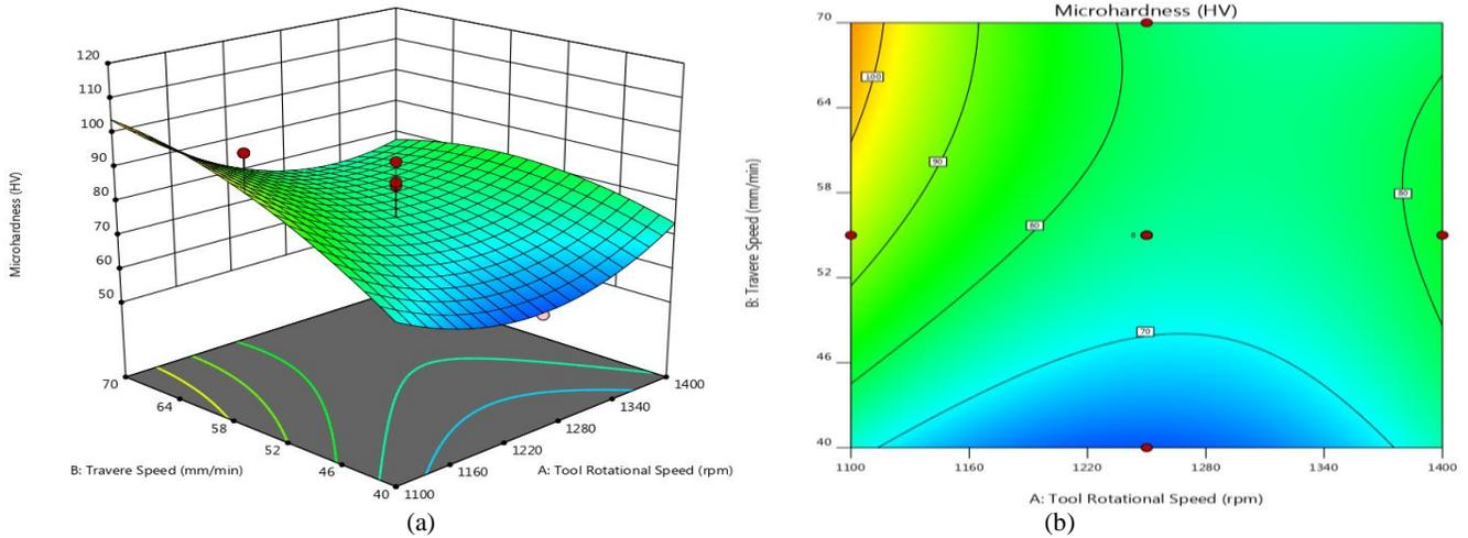
Figure 6: Effect of tool rotational speed and traverse speed on micro-hardness of friction stir welded joint
