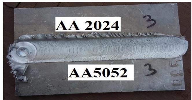
Figure 2: Friction stir welded joint of AA5052 and AA2024
