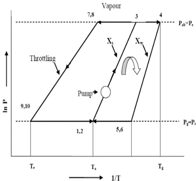
Figure 2.b: Single effect vapour absorption Refrigeration cycle on log p-1/T coordinates.
