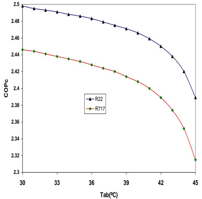
Figure 6: Variation in coefficient of performance with varying absorber temperature for different refrigerants at  $T_e=30^{\circ}\text{C}$ ,  $T_{w2}=85^{\circ}\text{C}$ ,  $T_c=35^{\circ}\text{C}$ ,  $T_{eva}=7^{\circ}\text{C}$ ,  $\text{Effectiveness}_{HE}=0.8$ ,  $\eta_c=0.85$ .
