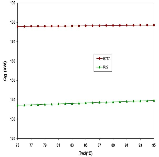
Figure 5: Variation of thermal load on Generator with varying cooling water inlet temperature for CHE for different refrigerants at  $T_e=30^{\circ}\text{C}$ ,  $T_{ab}=30^{\circ}\text{C}$ ,  $T_c=35^{\circ}\text{C}$ ,  $T_{eva}=7^{\circ}\text{C}$ ,  $\text{Effectiveness}_{HE}=0.8$ ,  $\eta_c=0.85$ .
