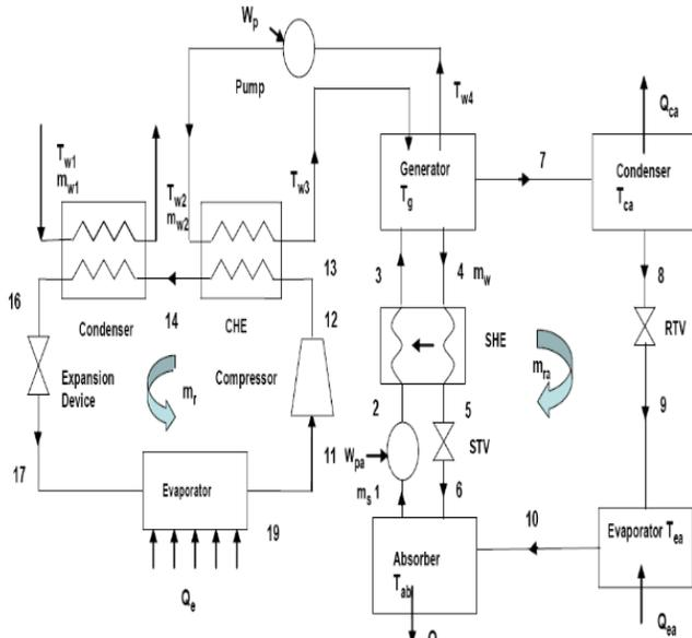
Figure 2.a Schematic diagram of an Integrated Refrigeration System (IRS)
