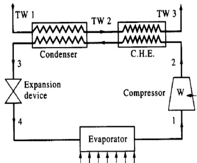
Figure 1: Vapour Compression refrigeration system
