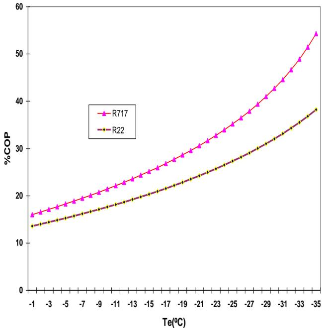
Figure 4: Variation in % increase in coefficient of performance with varying evaporator temperature For different refrigerants at  $T_{absorber}=30^{\circ}\text{C}$ ,  $T_{cond}=35^{\circ}\text{C}$ ,  $T_{eva}=7^{\circ}\text{C}$ ,  $T_{w2}=85^{\circ}\text{C}$ ,  $\text{Effectiveness}_{HE}=0.8$ ,  $\eta_c=0.85$ .
