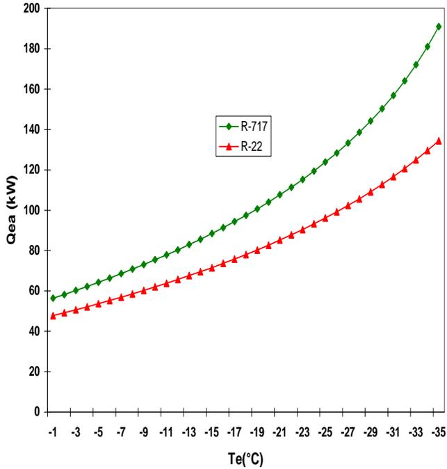
Figure 3: Heat added variations with evaporator of vapour absorption system by varying evaporator temperature of VCR for different refrigerants  $T_{absorber}=30^{\circ}\text{C}$ ,  $T_{condenser}=35^{\circ}\text{C}$ ,  $T_{eva}=7^{\circ}\text{C}$ ,  $T_{w2}=85^{\circ}\text{C}$ ,  $\text{Effectiveness}_{HE}=0.8$ ,  $\eta_c=0.85$
