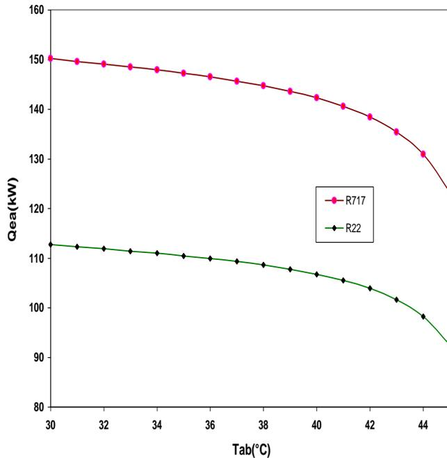
Figure 7: Variation in heat added to evaporator of VAR with varying absorber temperature for different refrigerants at  $T_{eva} = -30^{\circ}\text{C}$ ,  $T_{w2} = 85^{\circ}\text{C}$ ,  $T_{cond} = 35^{\circ}\text{C}$ ,  $T_{ea} = 7^{\circ}\text{C}$ ,  $\text{Effectiveness}_{HE} = 0.8$ ,  $\eta_c = 0.85$ .
