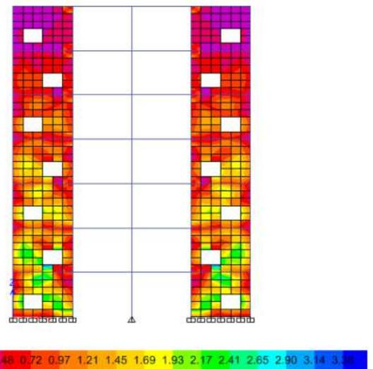
Figure 11: Stress distribution in shear wall with staggered openings
