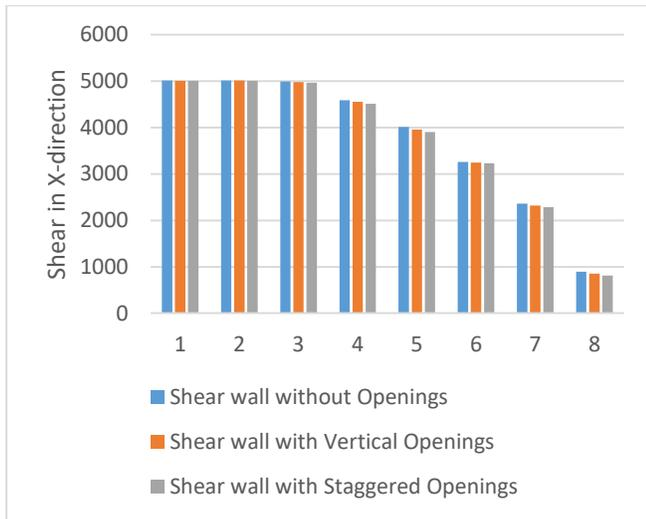
Figure 8: Story versus Story Shear in X-direction
