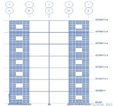
Figure 1: Elevation of the frame-shear wall building with vertical openings
