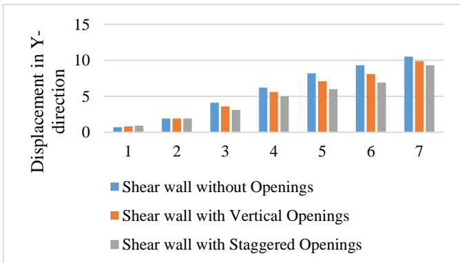
Figure 5: Story versus Story Displacement in Y-direction
