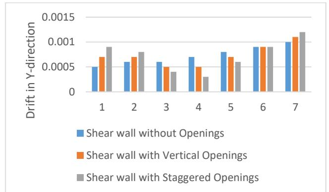
Figure 7: Story versus Story Drift in Y-direction
