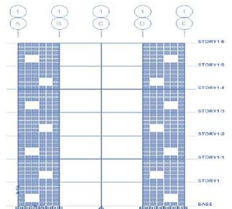
Figure 2: Elevation of the frame-shear wall building with staggered openings
