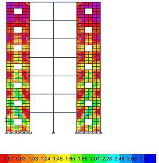
Figure 10: Stress distribution in shear wall with vertical openings
