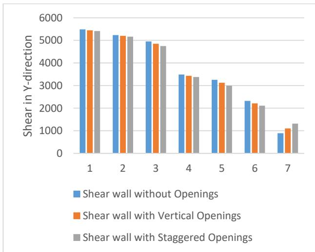
Figure 9: Story versus Story Shear in Y-direction
