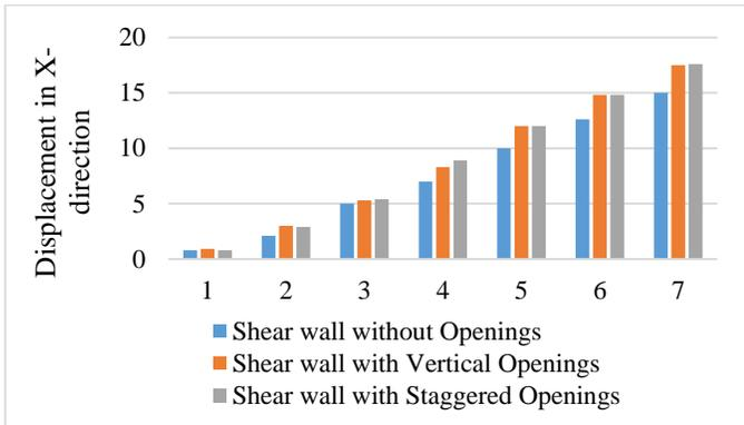
Figure 4: Story versus Story Displacement in X-direction
