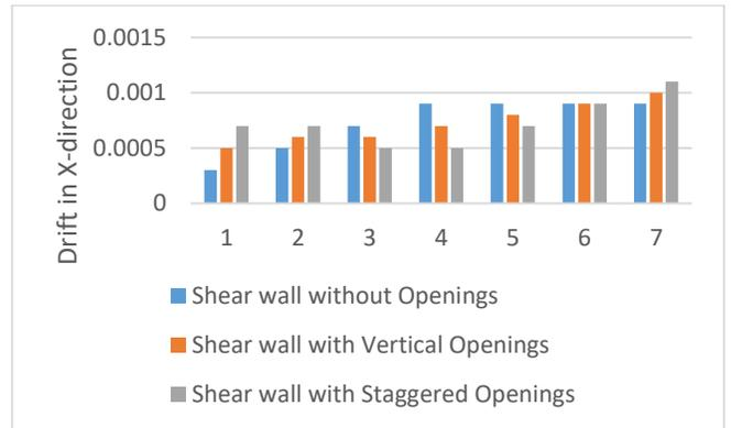
Figure 6: Story versus Story Drift in X-direction
