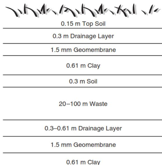
Figure 2: Typical cross-section of a landfill receiving MSW [32].
