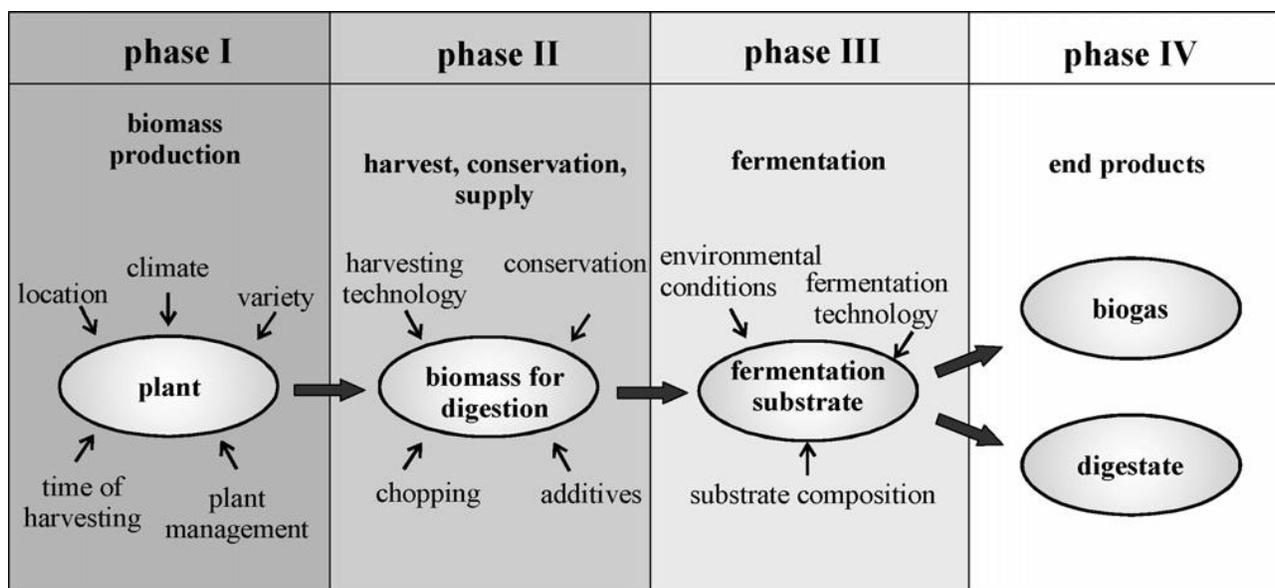
Figure 5: Effect on biogas production from maize along the production process [12].
