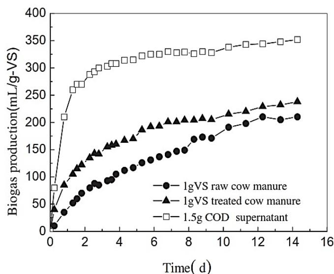
Figure 4: Cumulative biogas production of raw cow dung [11].
