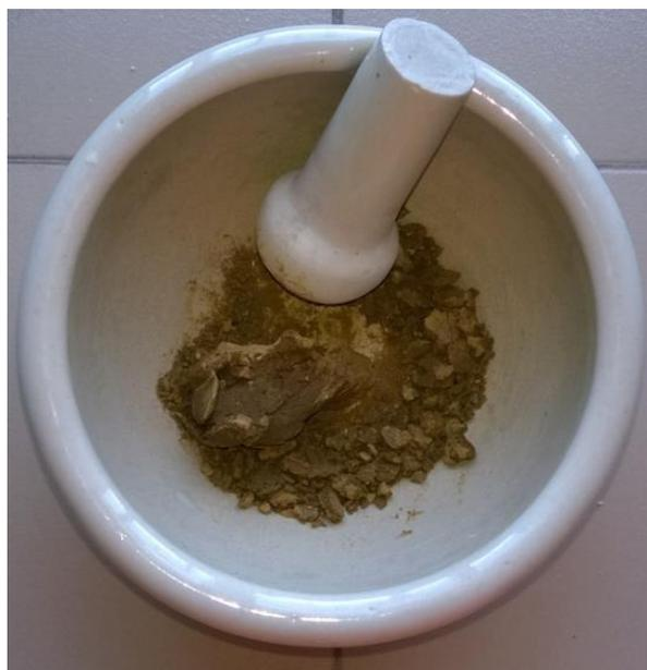
Figure 3. Crushing of dried clay samples
