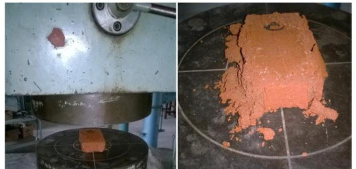
Figure 11. Measuring of compressive load of bricks
