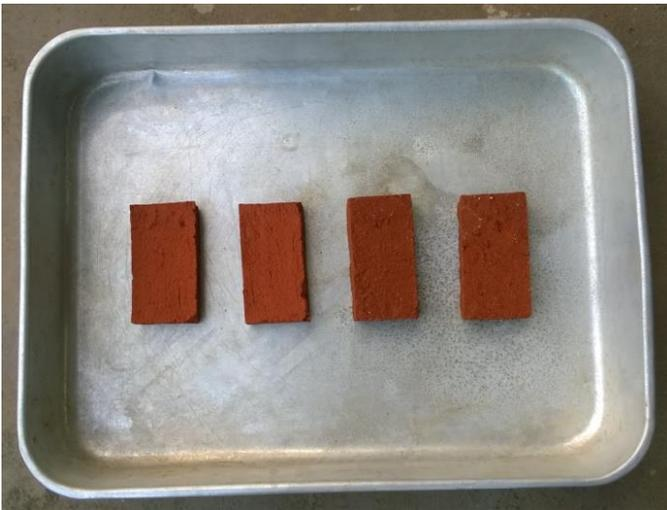
Figure 9. Manufactured bricks
