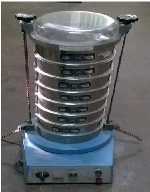
Figure 5. Apparatus setup for sieve analysis
