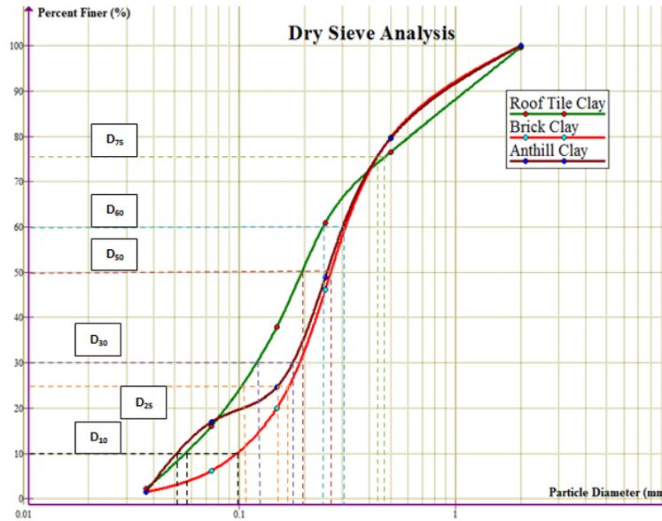
Figure 18. Particle size distribution curves of clays
