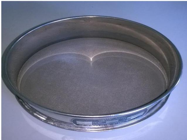
Figure 6. Sieve of 0.075mm
