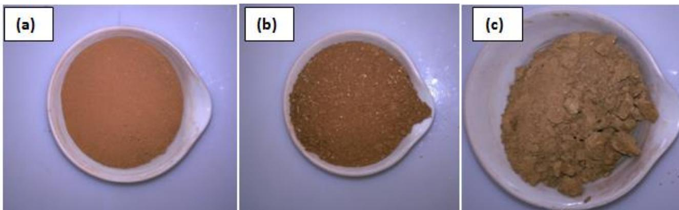
Figure 2. (a) Anthill clay, (b) brick clay and (c) roof tile clay samples
