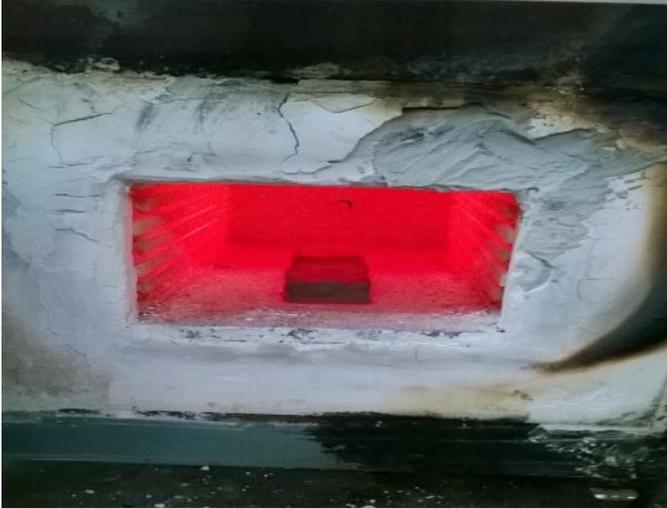
Figure 8. Firing of bricks using a muffle furnace
