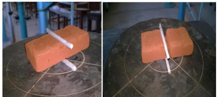
Figure 12. Measuring of splitting tensile load of bricks
