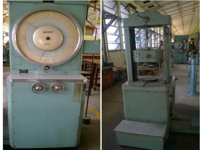
Figure 10. Universal tensile strength testing machine
