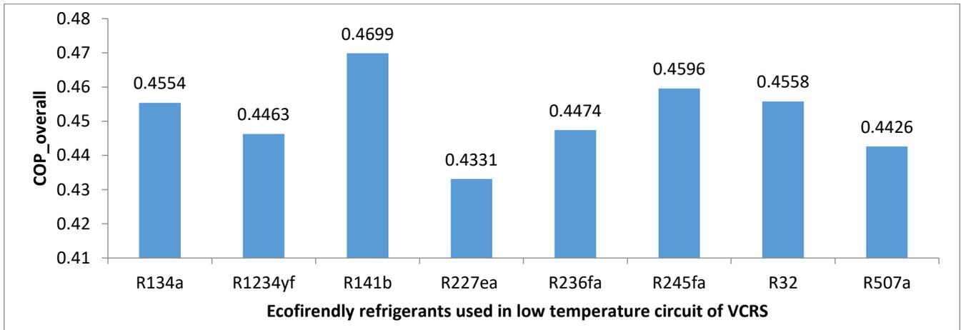
Figure 1: Thermal performances in terms of first law efficiency (overall COP\_Cascade) of cascade single effect ammonia-water ( $NH_3-H_2O$ ) vapour absorption refrigeration system coupled with vapour compression refrigeration using ecofriendly refrigerants in the low temperature cycle of VCRES system
