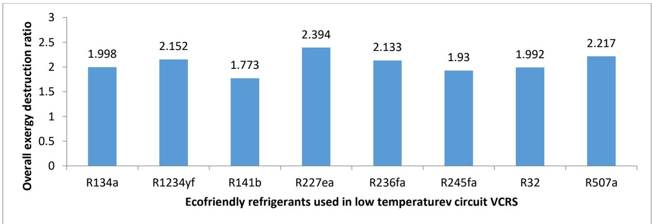
Figure 2: Thermal performances in terms of overall exergy destruction ratio (EDR\_Overall) of cascade single effect ammonia-water ( $NH_3-H_2O$ ) with vapour absorption refrigeration system coupled with vapour compression refrigeration using ecofriendly refrigerants in the low temperature cycle of VCRES system
