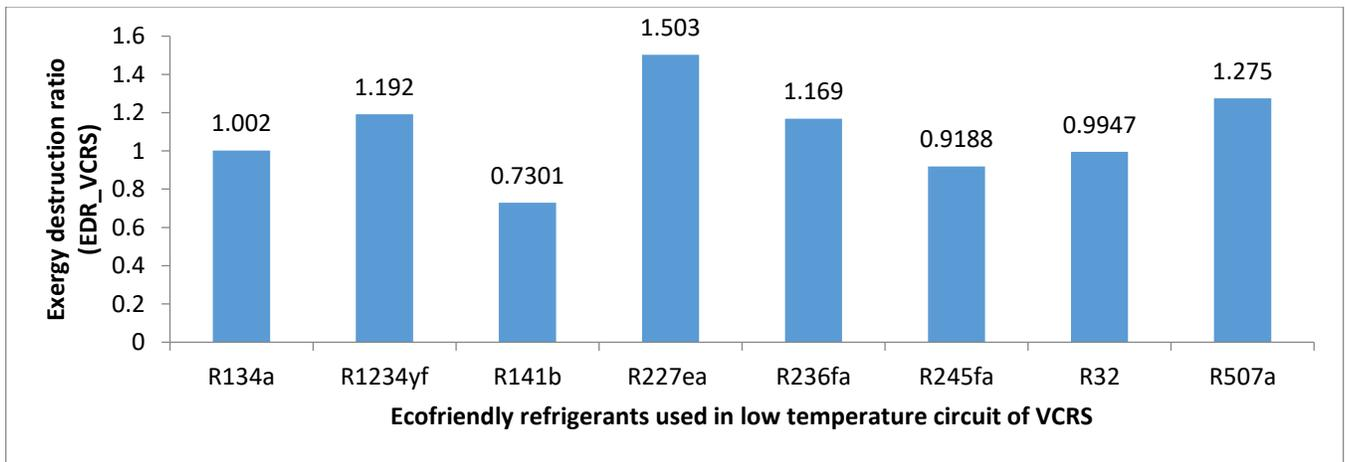
Figure 5: Thermal performances in terms of exergy destruction ratio (EDR\_VCERS) of vapour compression system of vapour compression refrigeration system (COP\_VCERS), of cascaded with single effect ammonia-water ( $\text{NH}_3\text{-H}_2\text{O}$ ) vapour absorption refrigeration system coupled with vapour compression refrigeration using ecofriendly refrigerants in the low temperature cycle of VCERS system
