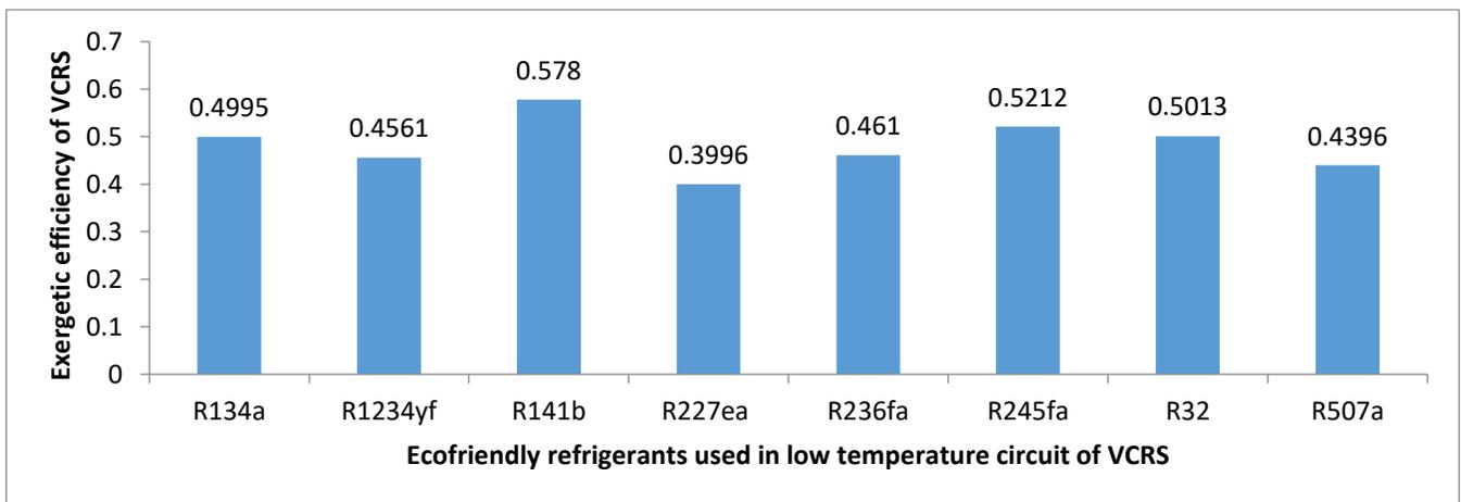
Figure 6: Thermal performances in terms of exergetic efficiency of vapour compression system of vapour compression refrigeration system (COP\_VCERS), of cascaded with single effect ammonia-water ( $\text{NH}_3\text{-H}_2\text{O}$ ) vapour absorption refrigeration system coupled with vapour compression refrigeration using ecofriendly refrigerants in the low temperature cycle of VCERS system
