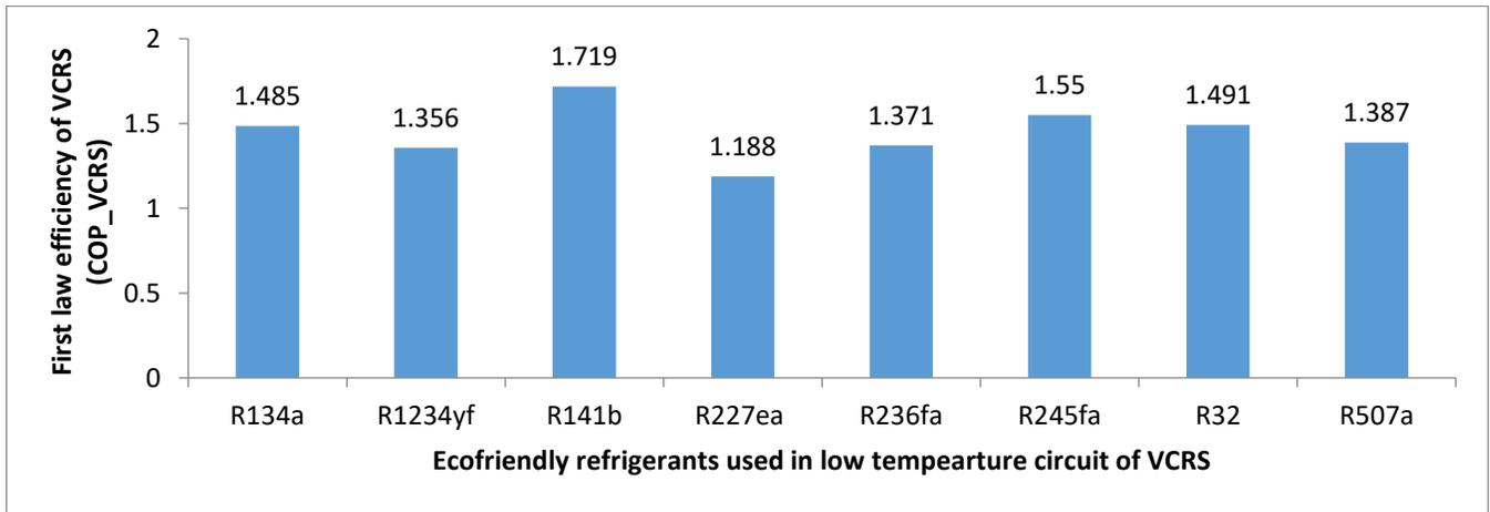
Figure 4: Thermal performances in terms of first law efficiency of vapour compression refrigeration system (COP\_VCERS) of cascaded with single effect ammonia-water ( $\text{NH}_3\text{-H}_2\text{O}$ ) vapour absorption refrigeration system coupled with vapour compression refrigeration using ecofriendly refrigerants in the low temperature cycle of VCERS system
