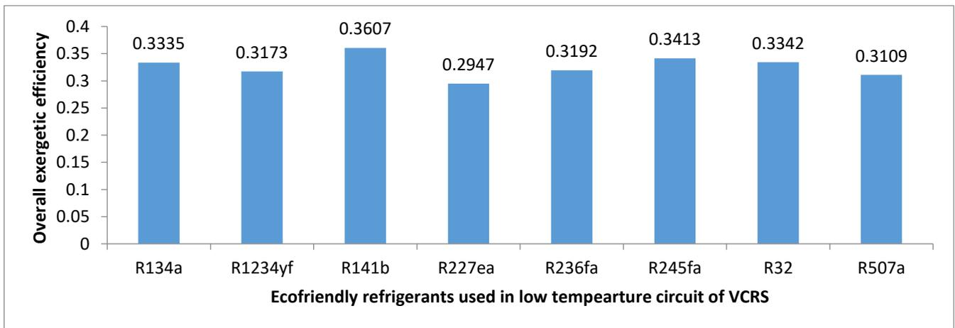
Figure 3: Thermal performances in terms of overall exergetic efficiency of cascaded single effect ammonia-water ( $NH_3-H_2O$ ) with vapour absorption refrigeration system coupled with vapour compression refrigeration using ecofriendly refrigerants in the low temperature cycle of VCRES system
