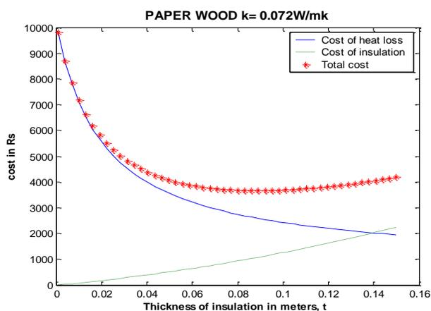
Figure 16b: Variation of total cost, cost of heat loss and cost of insulation with thickness of insulation for paper wood material
