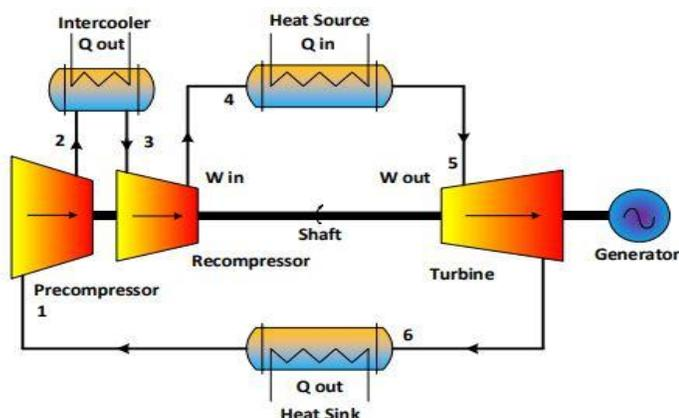
Figure 2: Brayton cycle with intercooling
