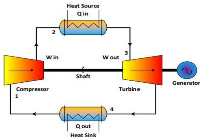
Figure 1: Schematic Diagram of Simple Brayton cycle
