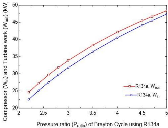
Fig 11 variation of compressor and turbine works with pressure ratio using R134a
