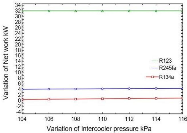
Fig 7 variation of net work of cycle with intercooler pressure
