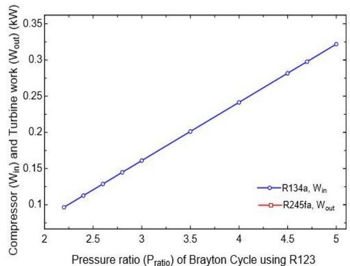
Fig 13 variation of compressor and turbine works with pressure ratio using R123
