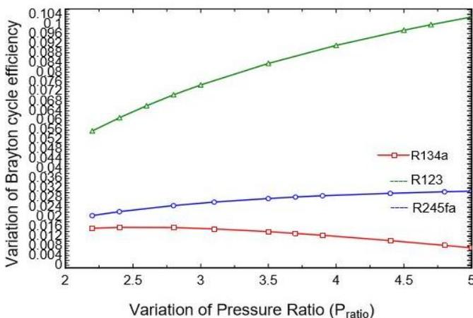
Fig 8 variation of cycle efficiency with pressure ratio
