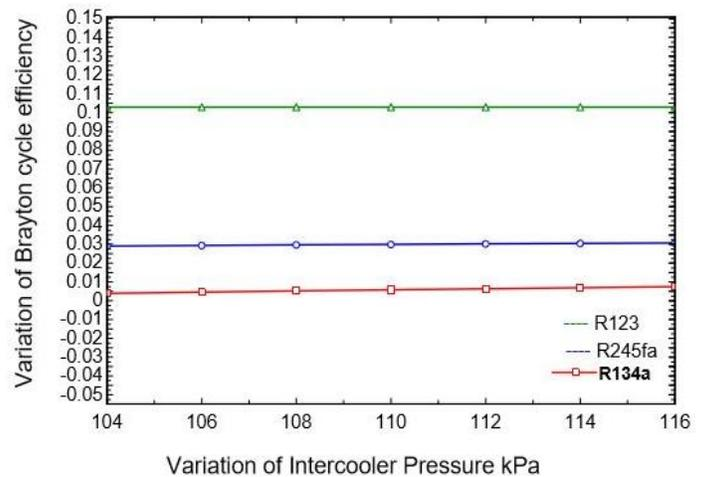
Figure 5: variation of cycle efficiency with intercooler pressure
