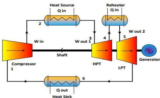
Figure 3: Layout of Brayton cycle with Reheating
