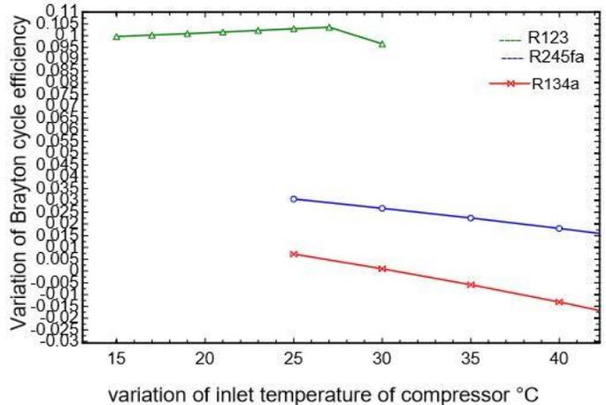
Fig 10 variation of Brayton cycle efficiency with inlet temperature of compressor
