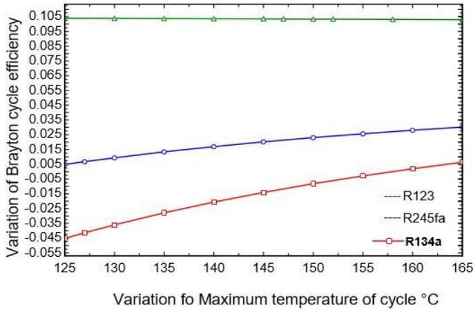
Fig 6 variation of cycle efficiency with maximum inlet temperature of turbine
