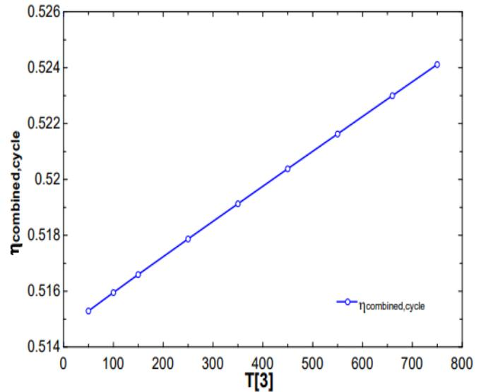
Figure 21: Variation between combined cycle efficiency and turbine inlet temperature of trans-critical Cycle.
