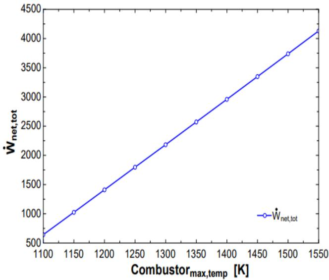
Figure 27: Variation between combined cycle net-work and cycle high temperature of Rankine Cycle
