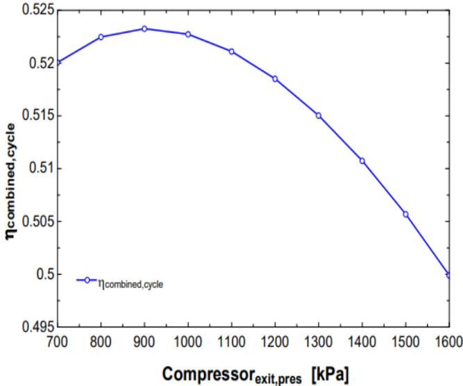
Figure 24: Variation between combined cycle efficiency and compressor exit pressure of Rankine Cycle
