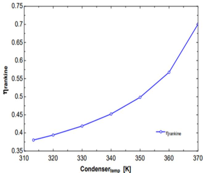
Figure 36: Variation between Rankine cycle efficiency and condenser temperature
