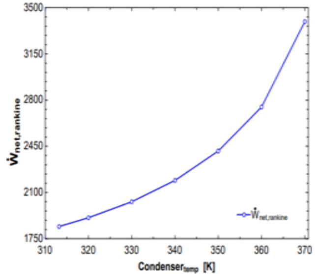
Figure 37: Variation between Rankine cycle net-work and condenser temperature.
