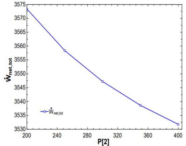
Figure 29: Variation between combined cycle net-work and exit pressure of pump of trans-critical cycle
