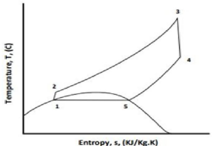
Figure 6: T-S Diagram of Trans-critical Cycle
