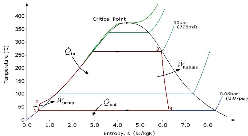
Figure 2: T-s diagram for Rankine cycle.
