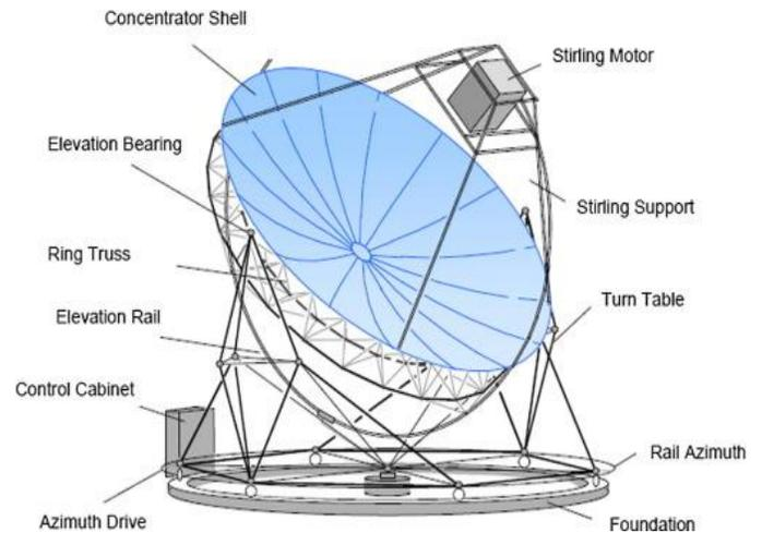
Figure 10: Parabolic dish-collector [25]
