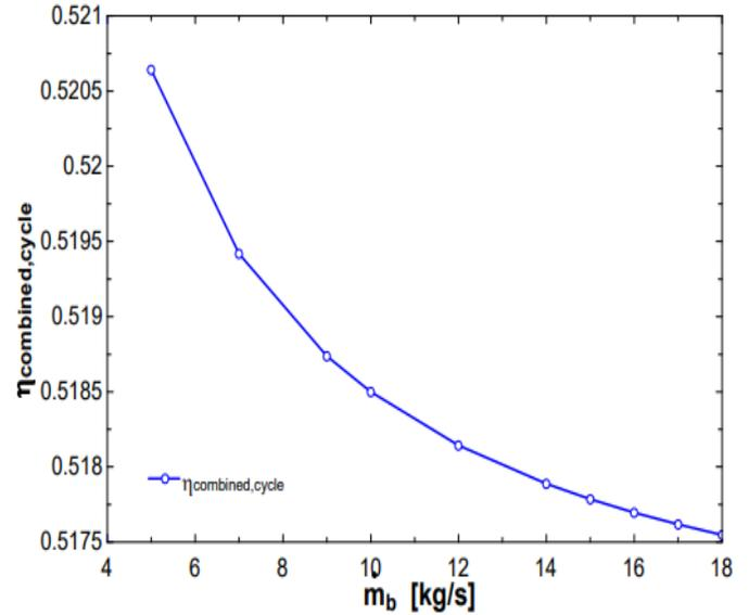
Figure 25: variation between combined cycle efficiency and mass flow rate of Brayton Cycle
