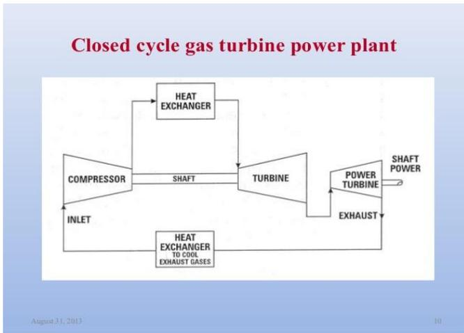
Figure 4: A closed-cycle gas turbine engine [4]
