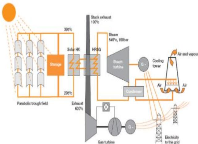
Figure 15: Integrated solar combined cycle [30]
