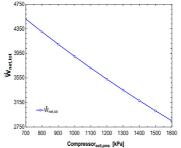
Figure 33: variation between combined cycle net-work and compressor exit pressure of Rankine Cycle
