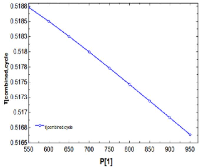
Figure 22: Variation between combined cycle efficiency and inlet pump pressure of trans-critical Cycle
