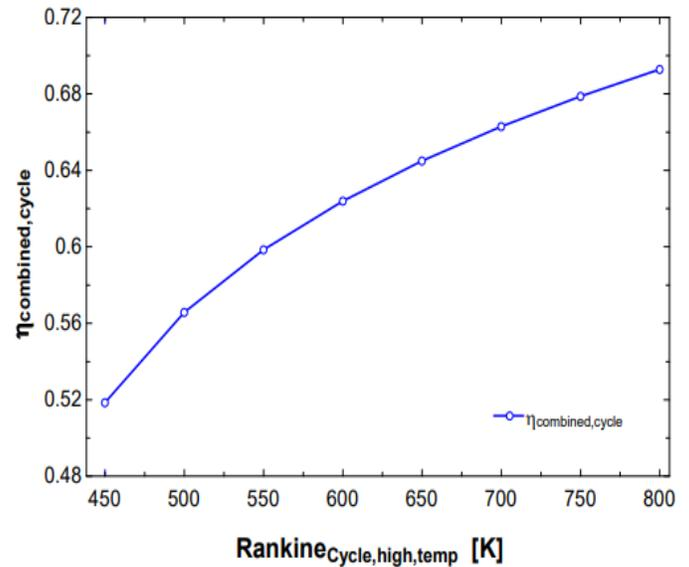
Figure 18: Variation between combined cycle efficiency and cycle high temperature of Rankine Cycle
