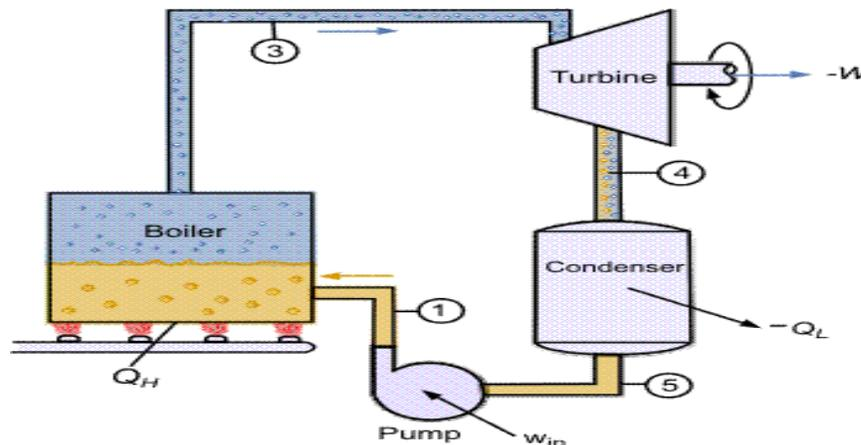
Figure 1: Basic design of Rankine cycle [1].
