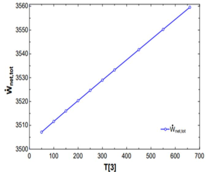
Figure 30: Variation between combined cycle net-work and turbine inlet temperature of trans-critical Cycle
