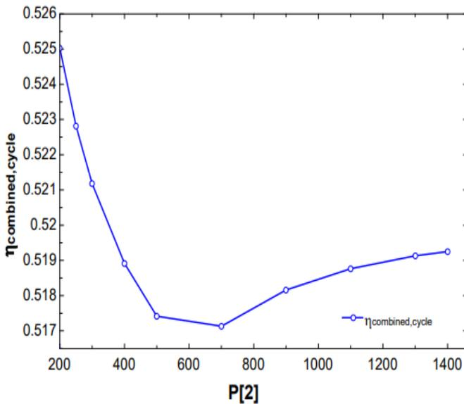
Figure 20: Variation between combined cycle efficiency and exit pressure of pump of trans-critical cycle.
