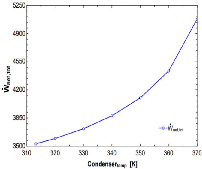
Figure 35: Variation between combined cycle net-work and condenser temperature of Rankine Cycle
