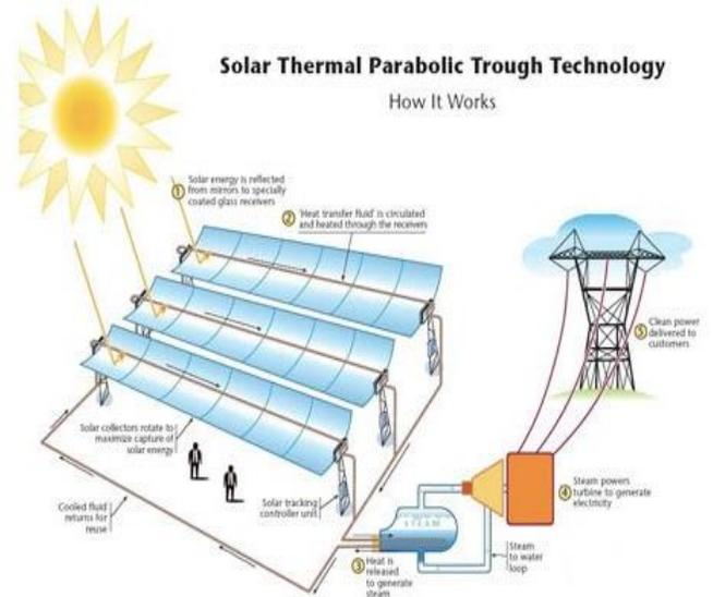
Figure 12: Parabolic trough system [27]
