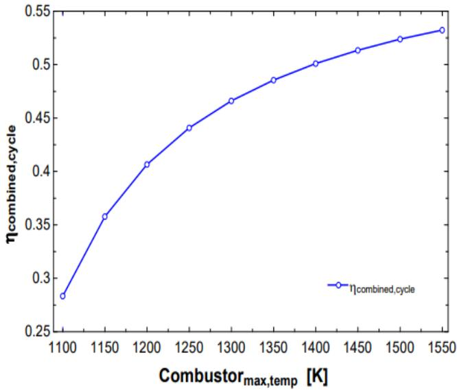
Figure 19: Variation between combined cycle efficiency and combustor maximum temperature of Brayton Cycle
