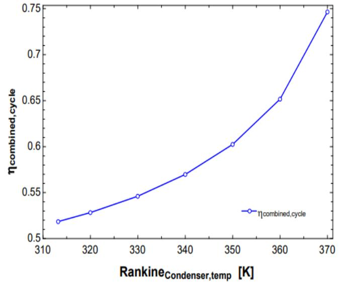
Figure 17: Variation between combined cycle efficiency and condenser temperature of Rankine Cycle
