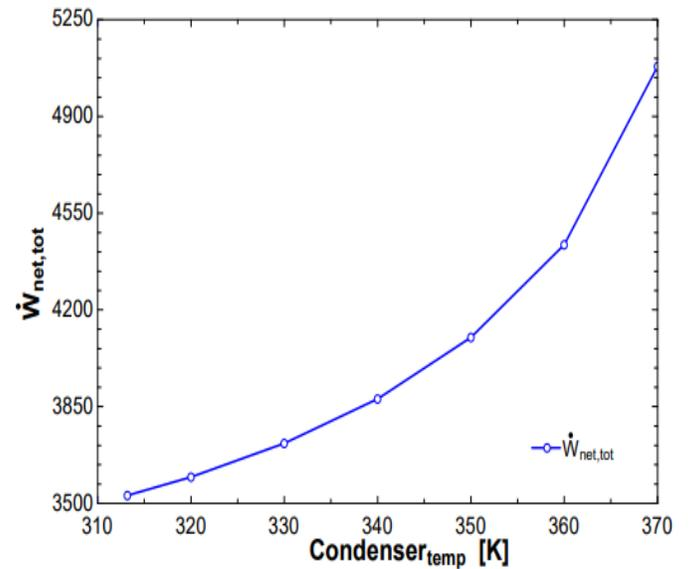
Figure 26: Variation between combined cycle net-work and condenser temperature of Rankine Cycle
