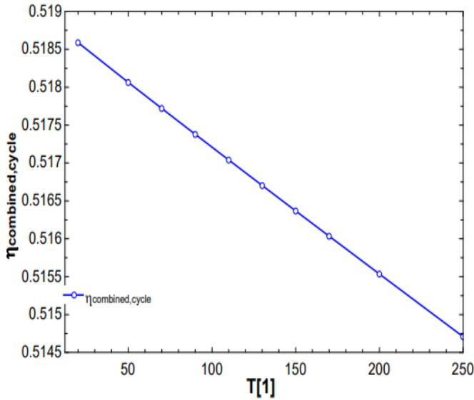
Figure 23: Variation between combined cycle efficiency and turbine inlet temperature of trans-critical Cycle
