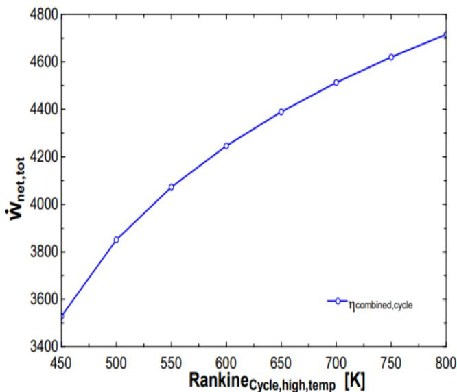
Figure 28: Variation between combined cycle net-work and combustor maximum temperature of Brayton Cycle
