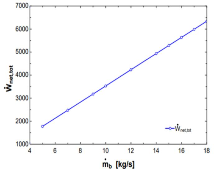
Figure 34: Variation between combined cycle net-work and mass flow rate of Brayton Cycle
