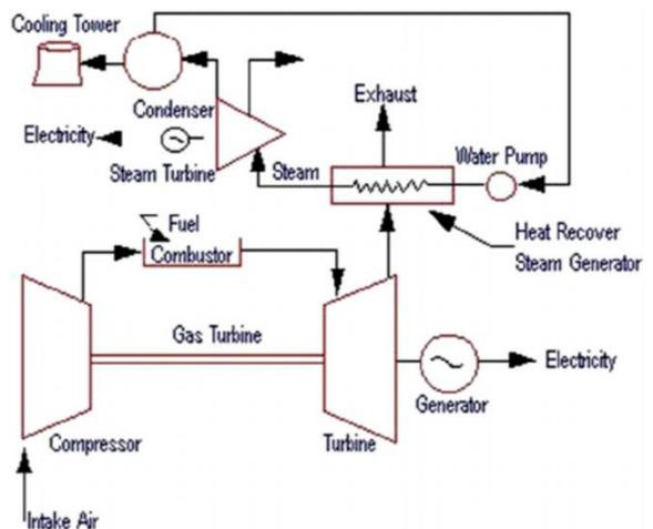
Figure 7: Combined Cycle Gas Turbine Plant HRSG [6]
