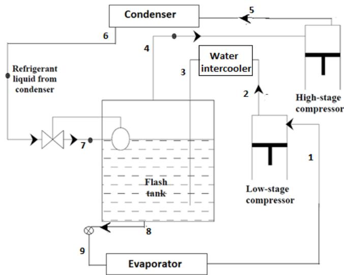
Figure 1: Two-stage vapour compression refrigeration system
