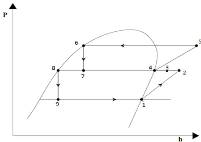
Figure 2: Pressure enthalpy diagram of two-stage VCRS
